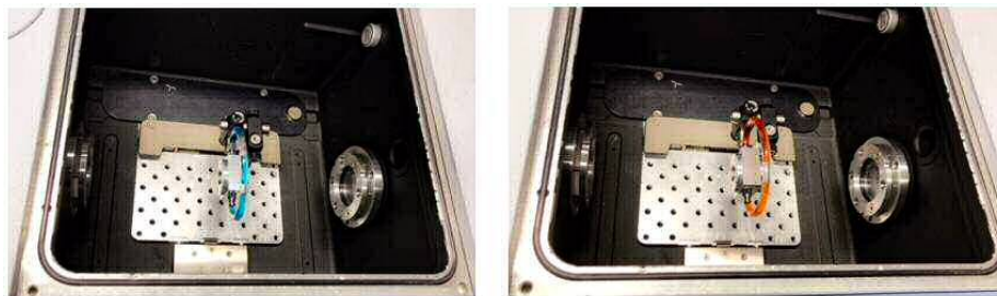
Figure 4.6: 0.01 mMol of each solution MB (left), and MO (right) in the Bruker Vertex 80V FTIR to identify and analyse the absorbance spectra of both of them
