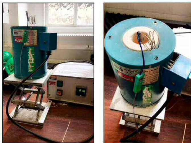
Figure 6.10: Rutile on the silicon wafer was calcined at 800 °C
