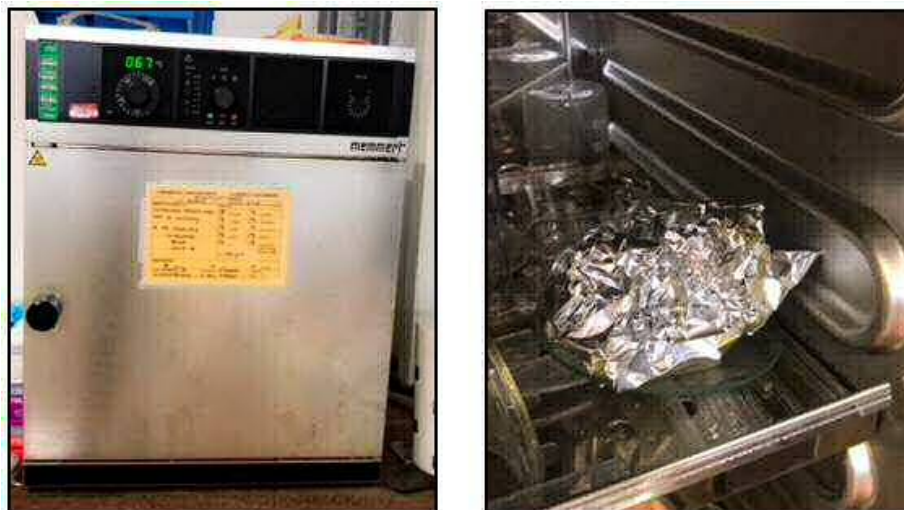
Figure 6.6: The precipitate in aluminium paper inside the oven to dry
