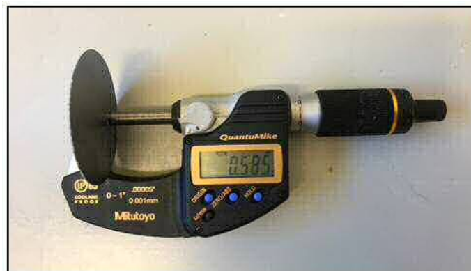
Figure 3.11: Thickness measurement of a stack of two wafers with coating
