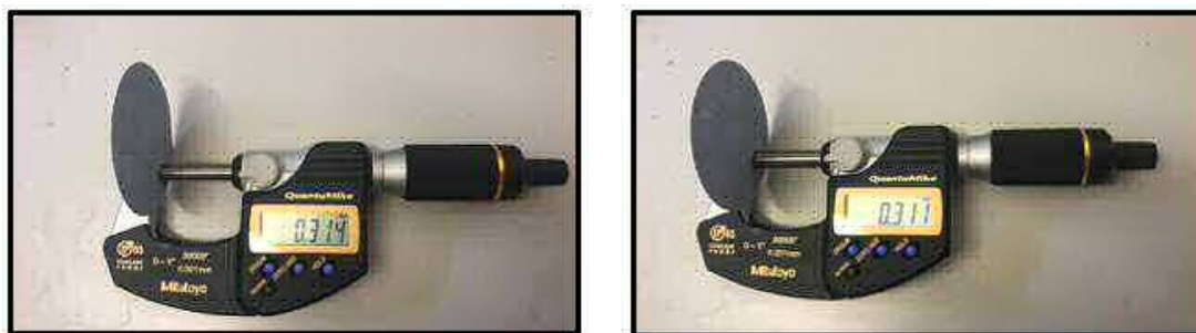
Figure 3.9: The different thicknesses of coated silicon wafer with \text{TiO}_2 nanoparticles
