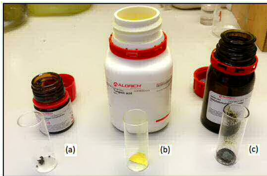
Figure 6.13: Desired mass of the dopants : (a) 0.0161g of Chromium (VI) nitrate \text{Cr}(\text{NO}_3)_6 , (b) 0.0169g of Tungstic acid \text{H}_2\text{WO}_4 , and (c) 0.0133 g of Molybdenum (V) pentachloride \text{MoCl}_5 .
