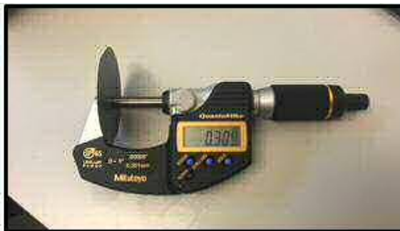
Figure 3.8: The thickness of a clean silicon wafer without any coating
