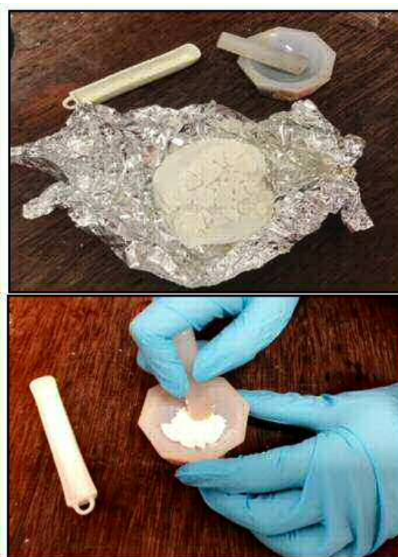
Figure 6.7: The upper image shows the shape of precipitate after drying it under 65 -70 degree while the bottom image shows the sample being grounded to become fine powder
