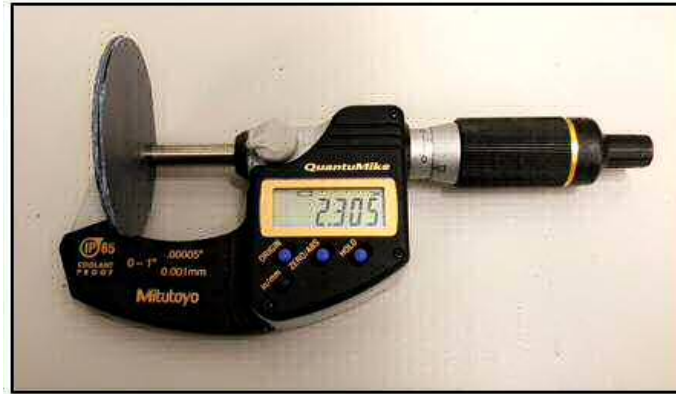
Figure 3.13: Thickness measurement of a big stack of six wafers with coating
