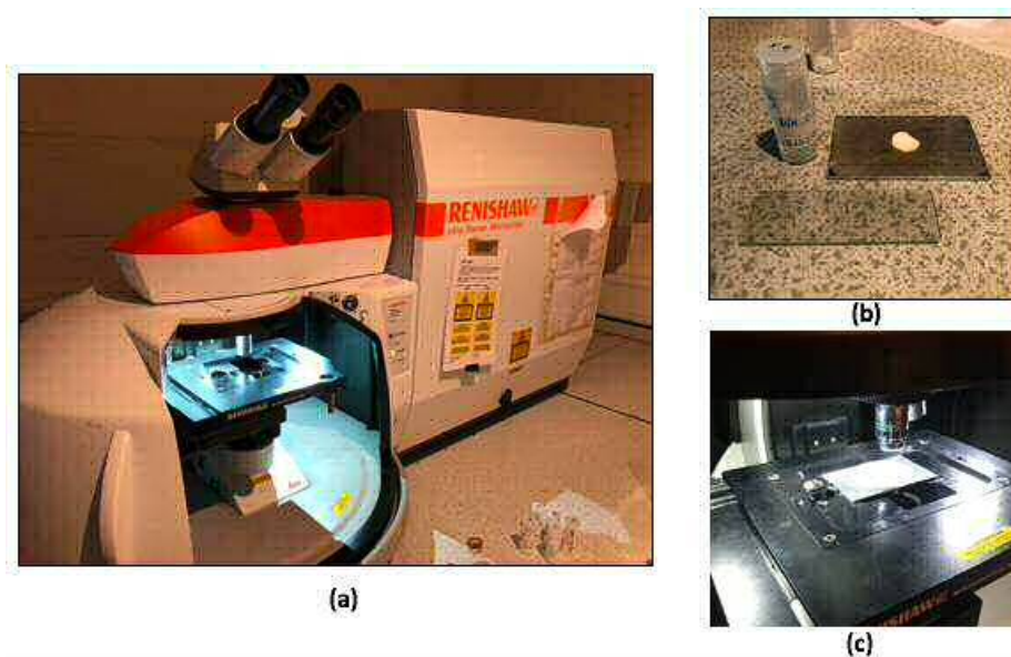
Figure 6.48: (a) Renishaw InVia Reflex Raman Spectrometer, (b) The sample (powder) to be examined, and (c) Coated wafer.
