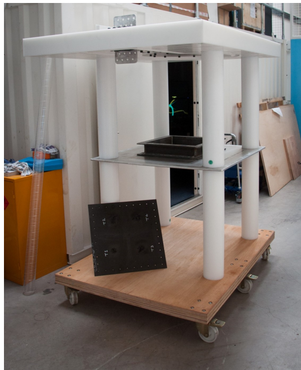
Figure 34 – Designed and constructed coaxial test rig
