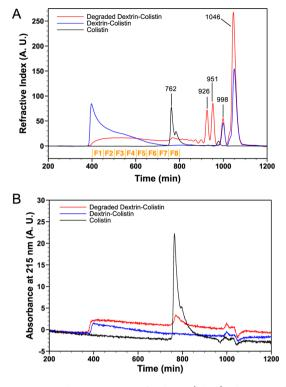
**Figure 2.** SEC chromatograms of colistin (black), dextrin–colistin conjugate (blue), and  $\alpha$ -amylase-treated (48 h at 37 °C) dextrin–colistin conjugate (red) by (A) RI detection and (B) UV detection ( $\lambda$  = 215 nm). Collected fractions are shown in orange.
