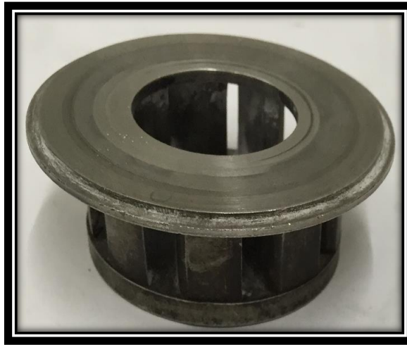
Figure 3.14 Tangential swirl configuration
