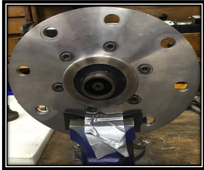
Figure 3.16 Diffusive injector centrally positioned in configuration
