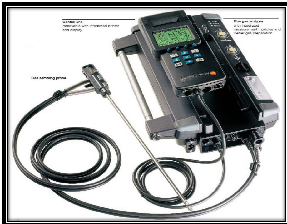
Figure 3.22 Testo 350 XL including analyser unit, control unit and gas probe
