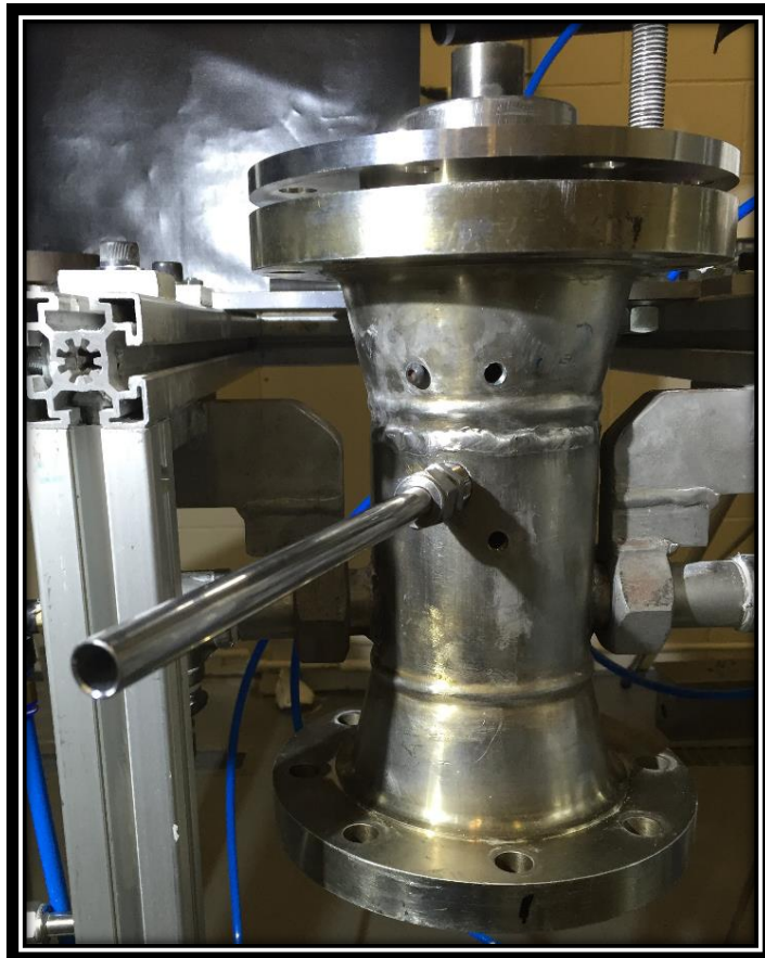
Figure 3.17 Fuel pipeline installed in burner
