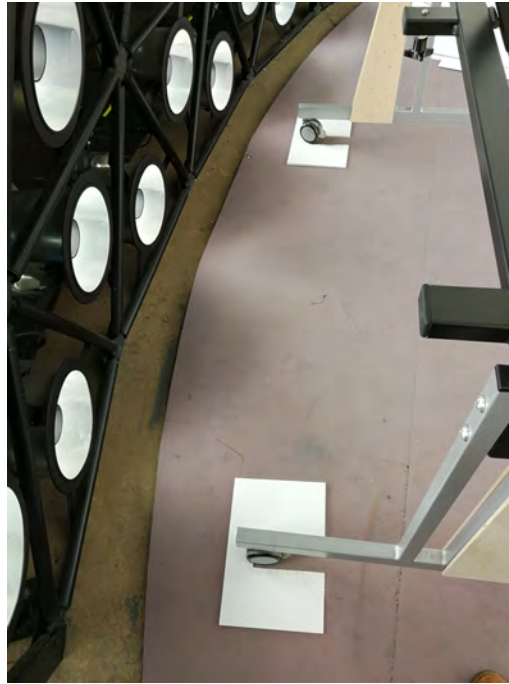
Figure 3.36: Masks on the floor to mark wheels positioning.
