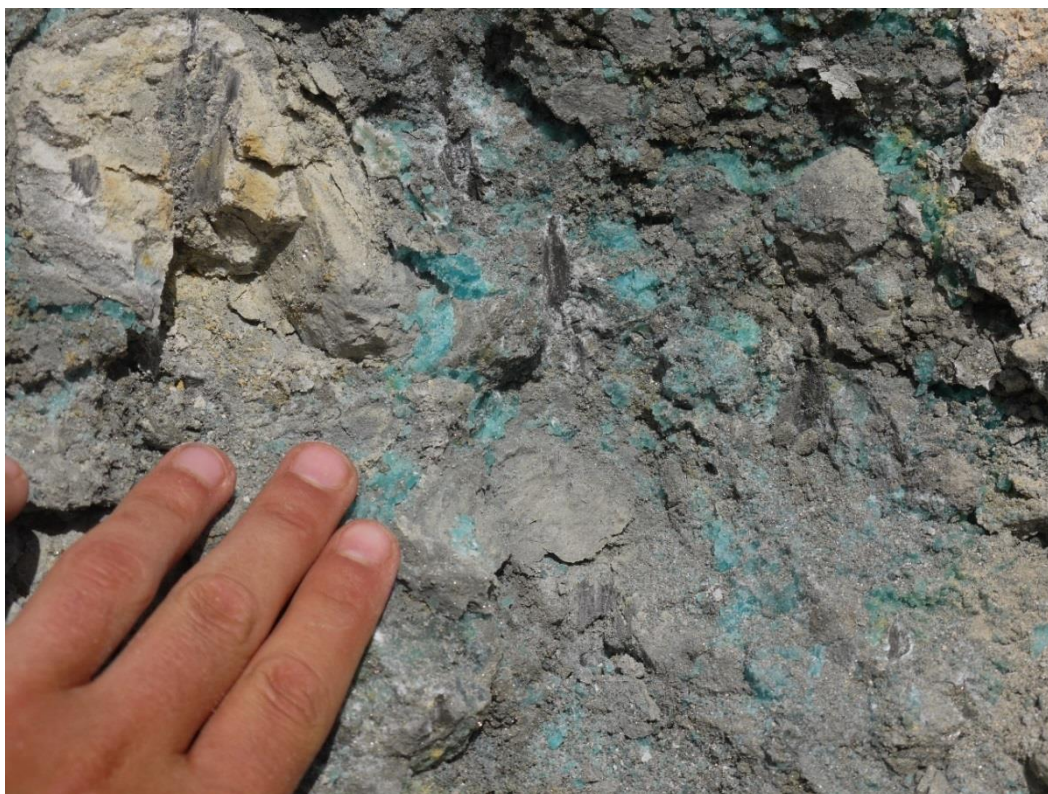
Figure A3.96: Typical gossan exposure. Multiple layers of Fe oxides and sulfates, predominantly jarosite, goethite and hematite.
