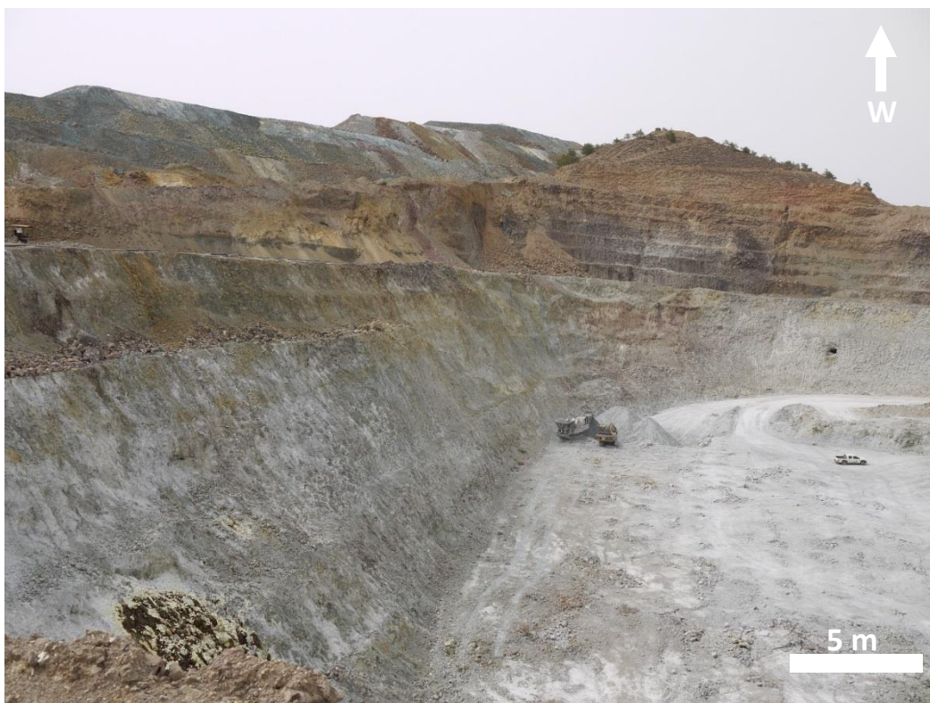
Figure A3.5: Cut and blast operation at Three Hills.
