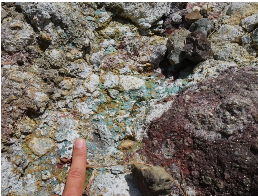
Figure A3.18: South Apliki Breccia zone mineralisation, hematite with disseminated pyrite, chalcopyrite and oxidised semi-massive ore.
