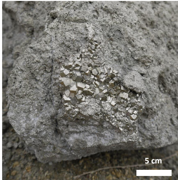
Figure A3.75: Massive euhedral pyrite (pyritohedrons).
