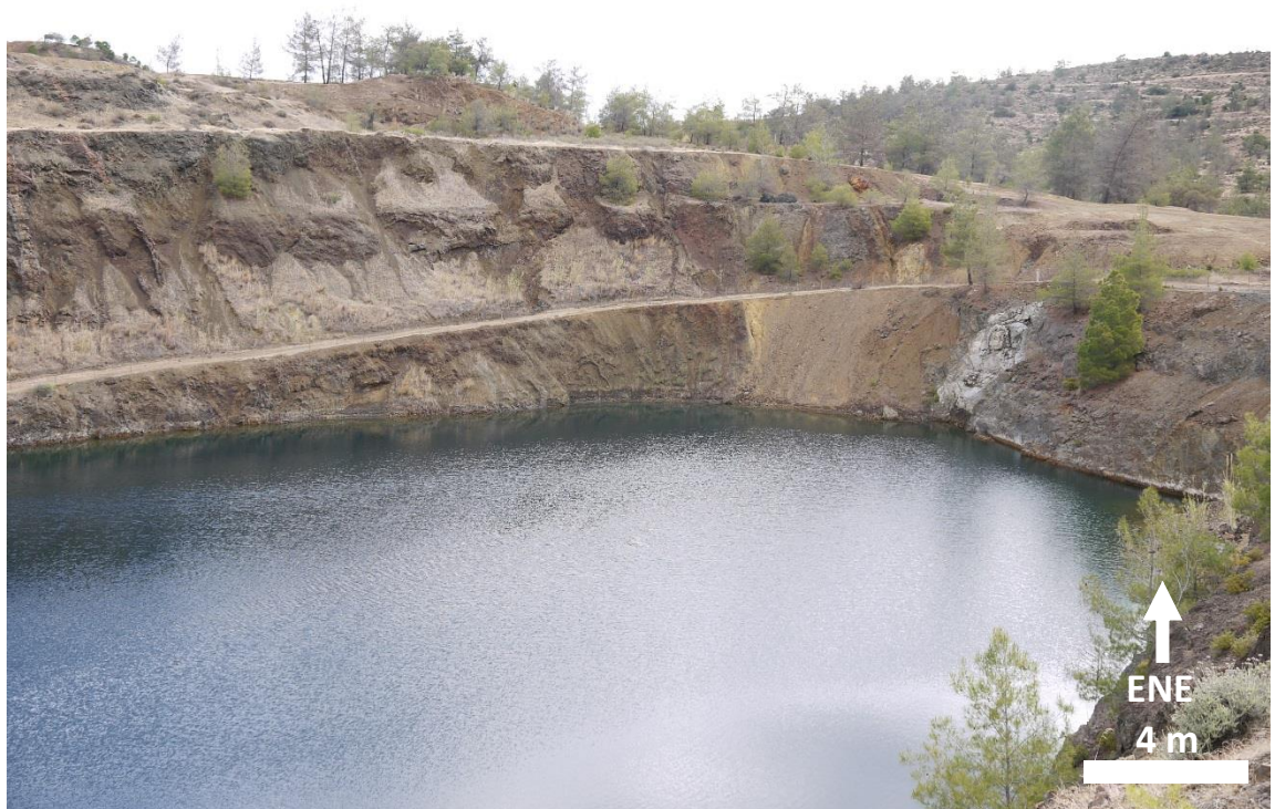
Figure A3.59: Fault zone in eastern pit margin. Increased leaching and oxidisation.
