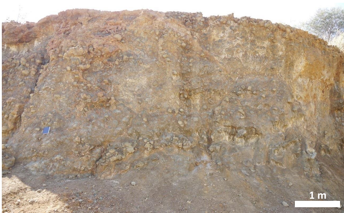
Figure A3.32: SE pit wall/corner. Cobbled, silicified boulders. Very highly silicified with disseminated pyrite. Cobbles are generally small (<30 cm) and highly spherical. They do not have chilled margins. Cobbled appearance is a function of preferential weathering of the exposed face.
