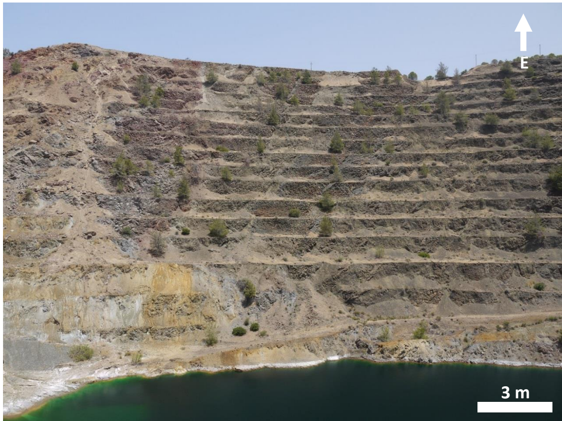
Figure A3.22: View of E pit wall. The boundary between the mineralised and non-mineralised LPL is distinct. The flows are ~1 m thick or less and dip at 40N/084.
