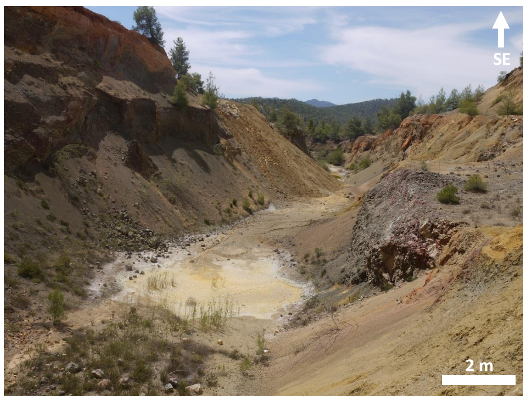
Figure A3.34: View along strike of major W fault. Foreground is “main” mineralisation with a pod of massive oxidised pyrite. The left wall is massive flows overlain by gossan. The area highlighted is the sharp transition from fragmented basalts with calcite matrix infill.
