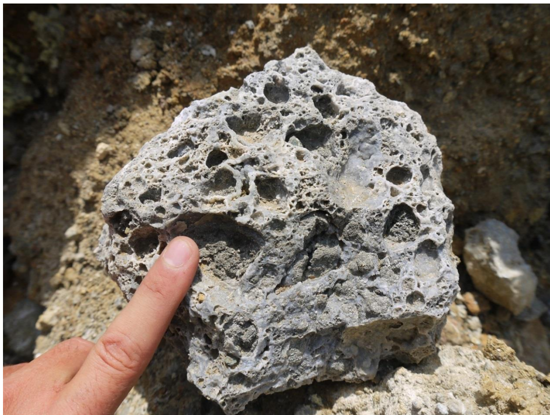
Figure A3.16: Silicified box-work texture with minor pyrite. Commonly found in the S pit area in distal mound areas. Voids suggest late dissolution (similar to Mathiatis N).
