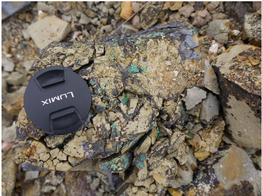
Figure A3.90: 'Unaltered' lava from lava dome with malachite and gypsum along contact.
