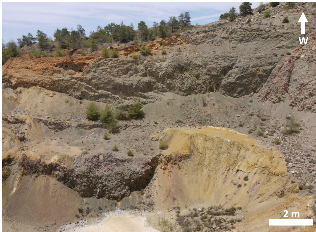
Figure A3.36: W pit wall. The limonitic mineralised horizon/UPL contact is clearly definable, it looks so sharp it could be erosional or seafloor topography covered by UPL? Gossan is well developed to the W. Note very sharp faulted boundary between LPL and UPL, downthrow to the N then infilling with UPL.
