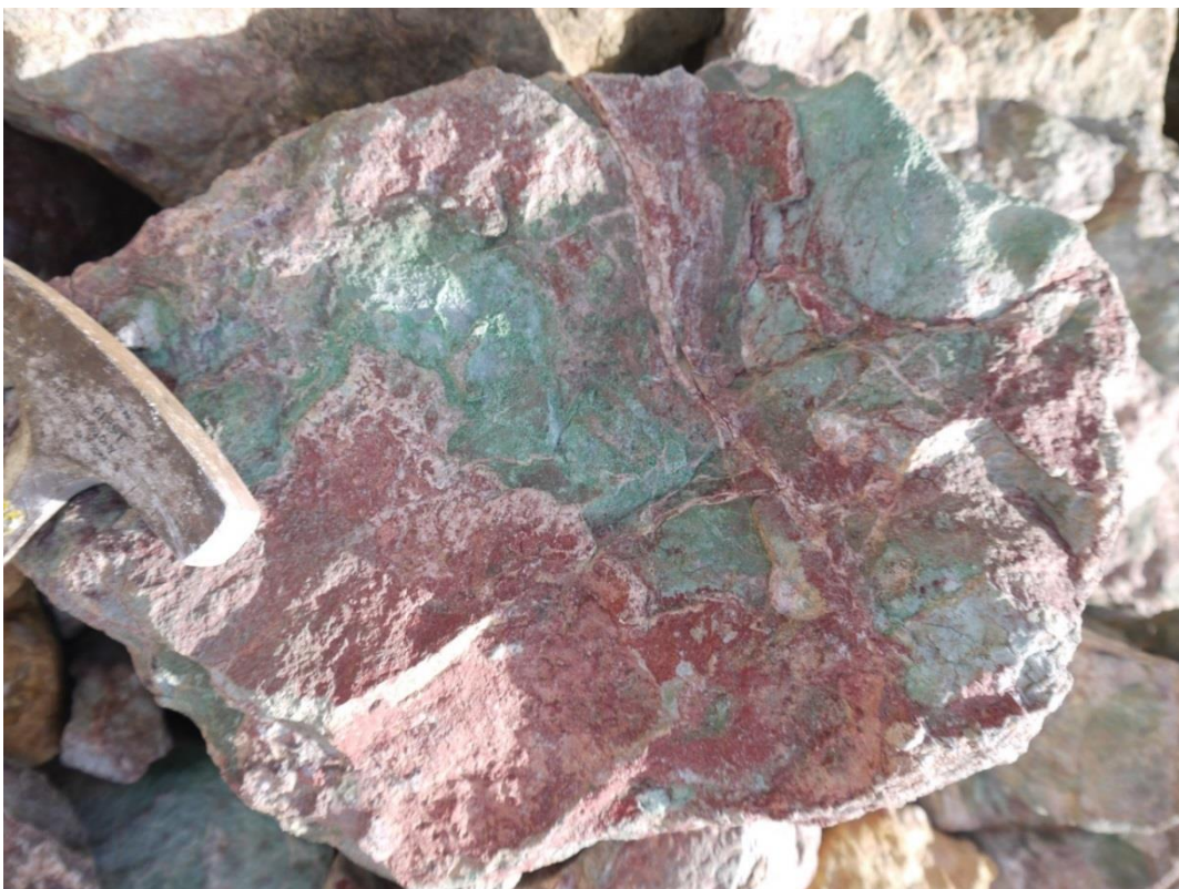
Figure A3.82: Typical wall-rock alteration. Hematite and chlorite with quartz veins.
