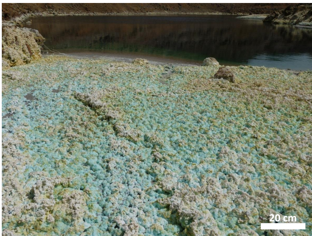
Figure A3.79: Copper sulfate precipitate at lake margin, the lake is uncharacteristically green in colour compared to the traditional deep red colour of a 'normal' VMS AMD.
