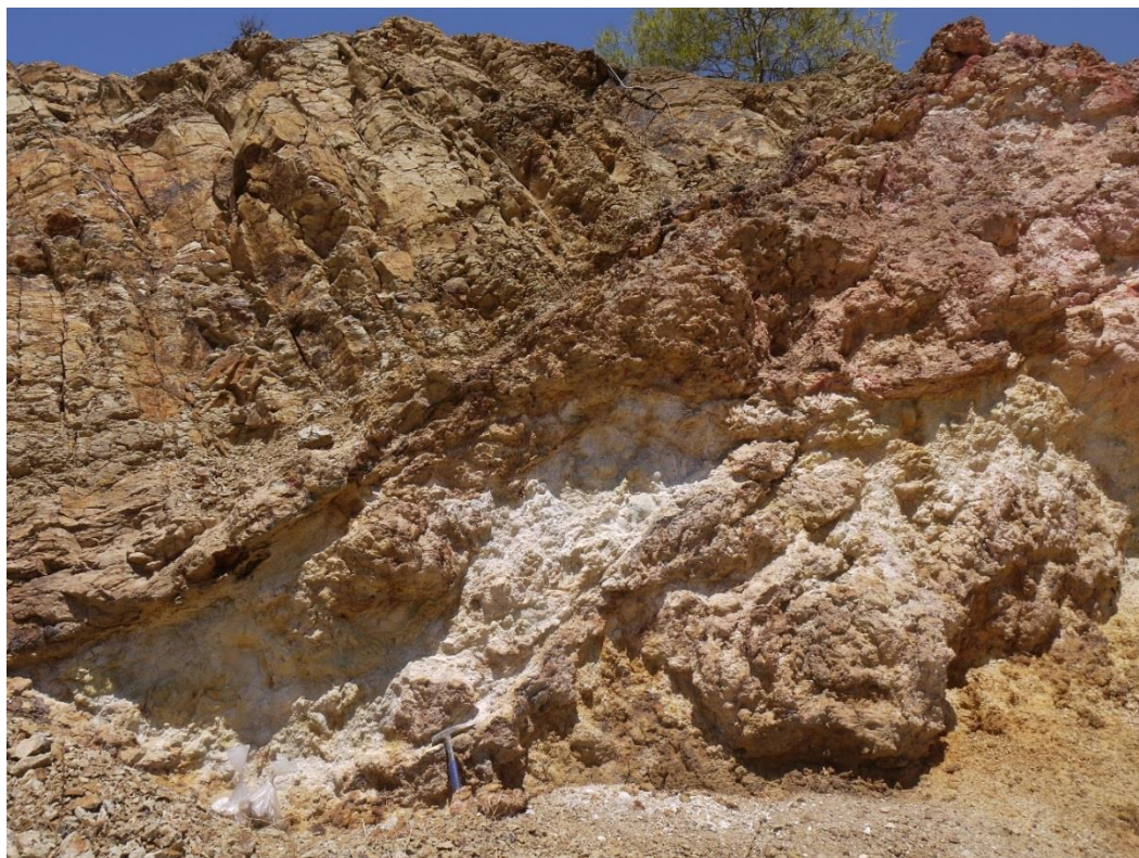
Figure A3.56: Fault contact between massive sulfide zone at N pit face. Upper (hanging wall) is massive un-altered flows exhibiting minor brecciation whilst the footwall is kaolinised and Fe stained.
