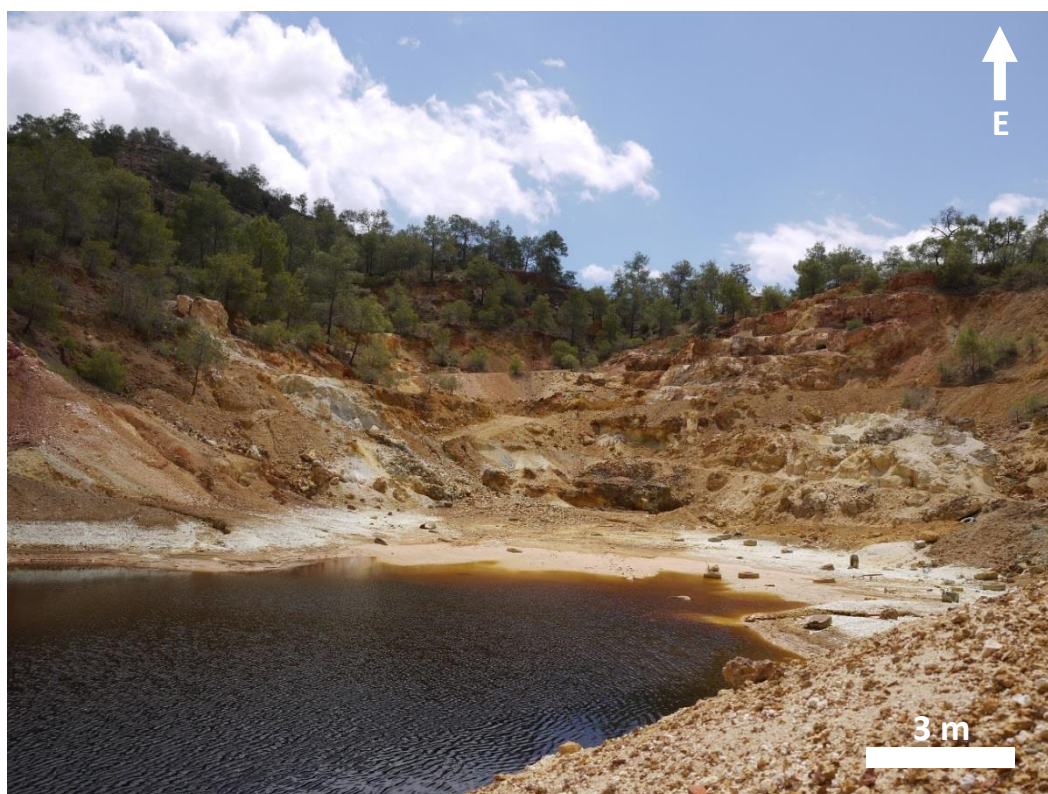
Figure A3.93: View over the Mathiatis open pit. Note the extensive gossan. AMD marks limit of historic mining for sulfide ore.
