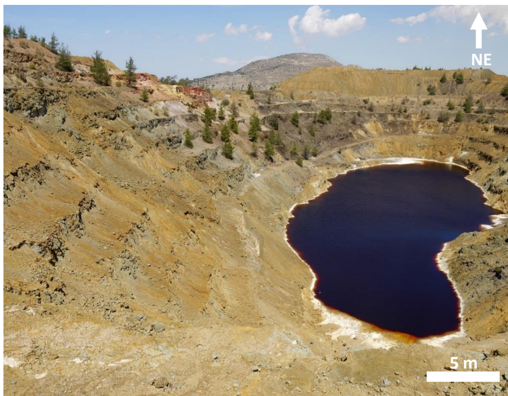
Figure A3.23: View of the Kokkinopezula pit. Note gossanised outcrop N. and wedge of darker UPL material in the central pit face. AMD is well developed.
