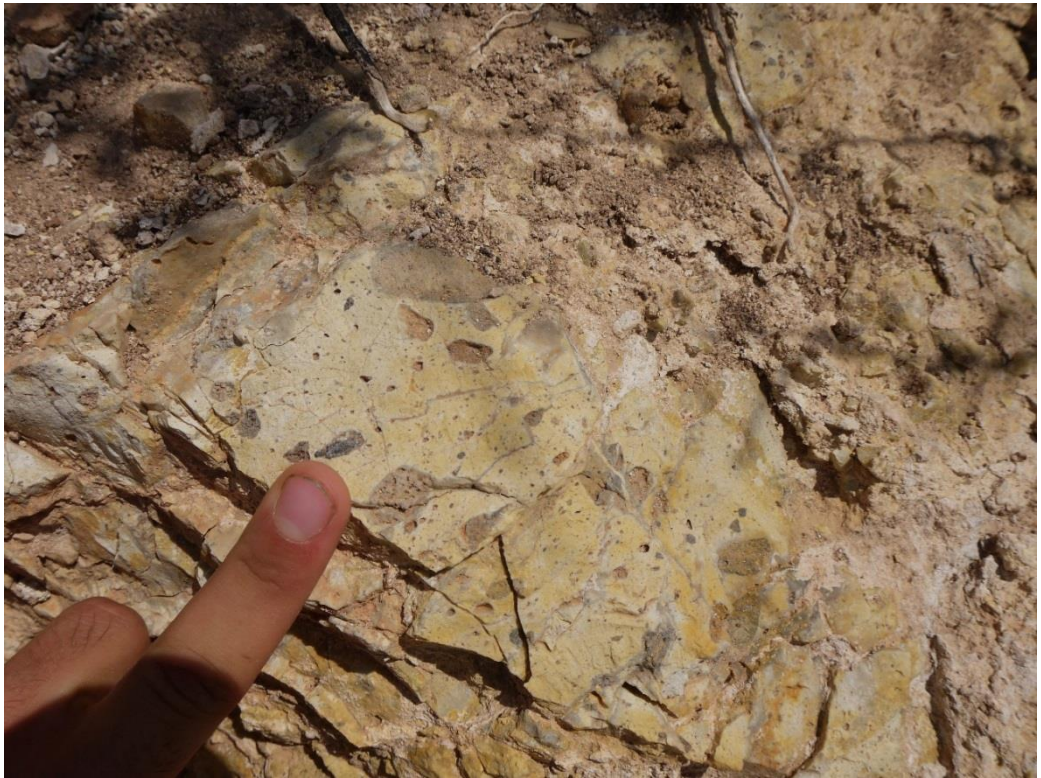
Figure A3.108: Rock with a pepperitic texture in the upper Touronjia area. Also contained minor disseminated pyrite.
