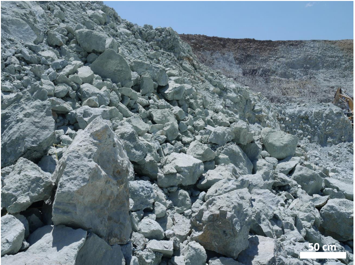
Figure A3.6: Typical Three Hills ore. Basalts are LPL and have been extensively chloritized. Ore occurs infilling fractures. A thin veneer of chalcopyrite with covellite + chalcocite. Pyrite is coarse (up to 1.5 cm) and euhedral.
