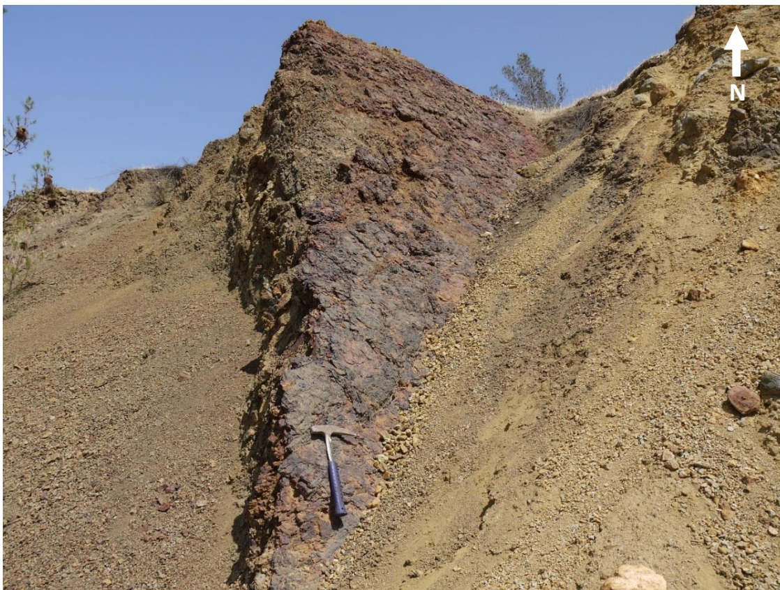
Figure A3.20: One of the main mineralising faults exposed at the top of the open pit (N side). Zone is highlighted by a breccia zone dipping 44E/002. The fault is responsible for the intense alteration of surrounding rocks in image above.
