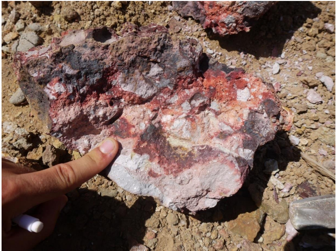
Figure A3.63: Typical breccia with hematite-pyrite matrix and sub-angular clasts.
