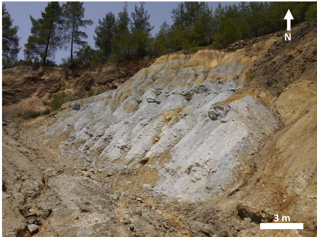
Figure A3.71: Massive sulfide mound NW Mala pit wall. Mound is homogenous massive pyrite with interstitial sulfate (<10%).
