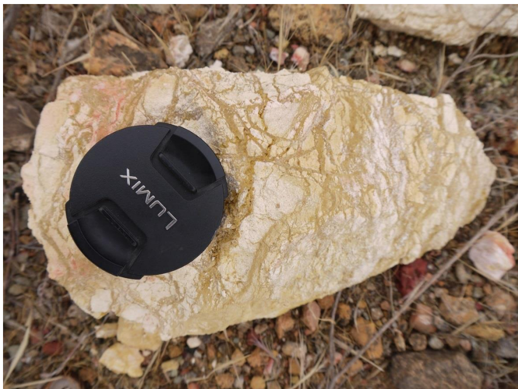
Figure A3.89: Veined hand specimen. Goethite veins in a leached silica-rich matrix.
