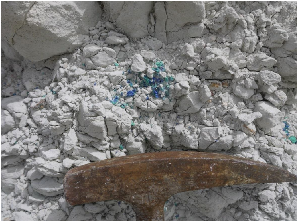
Figure A3.77: Highly bleached material with minor azurite and malachite.
