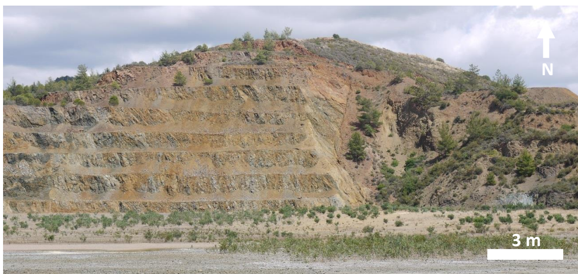
Figure A3.66: Main mineralising fault exposed in E pit corner. Footwall is heavily brecciated and Fe stained with disseminated sulfides.
