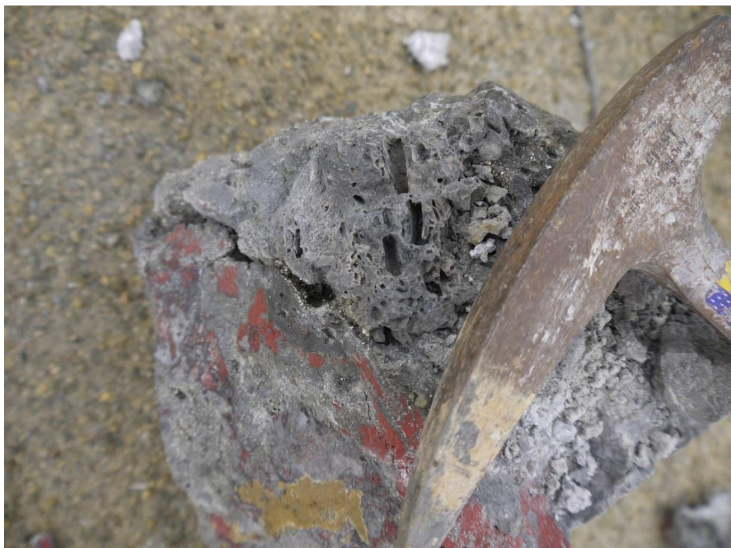
Figure A3.74: Jasper-stockwork vein exhibiting a boxy dissolution texture
