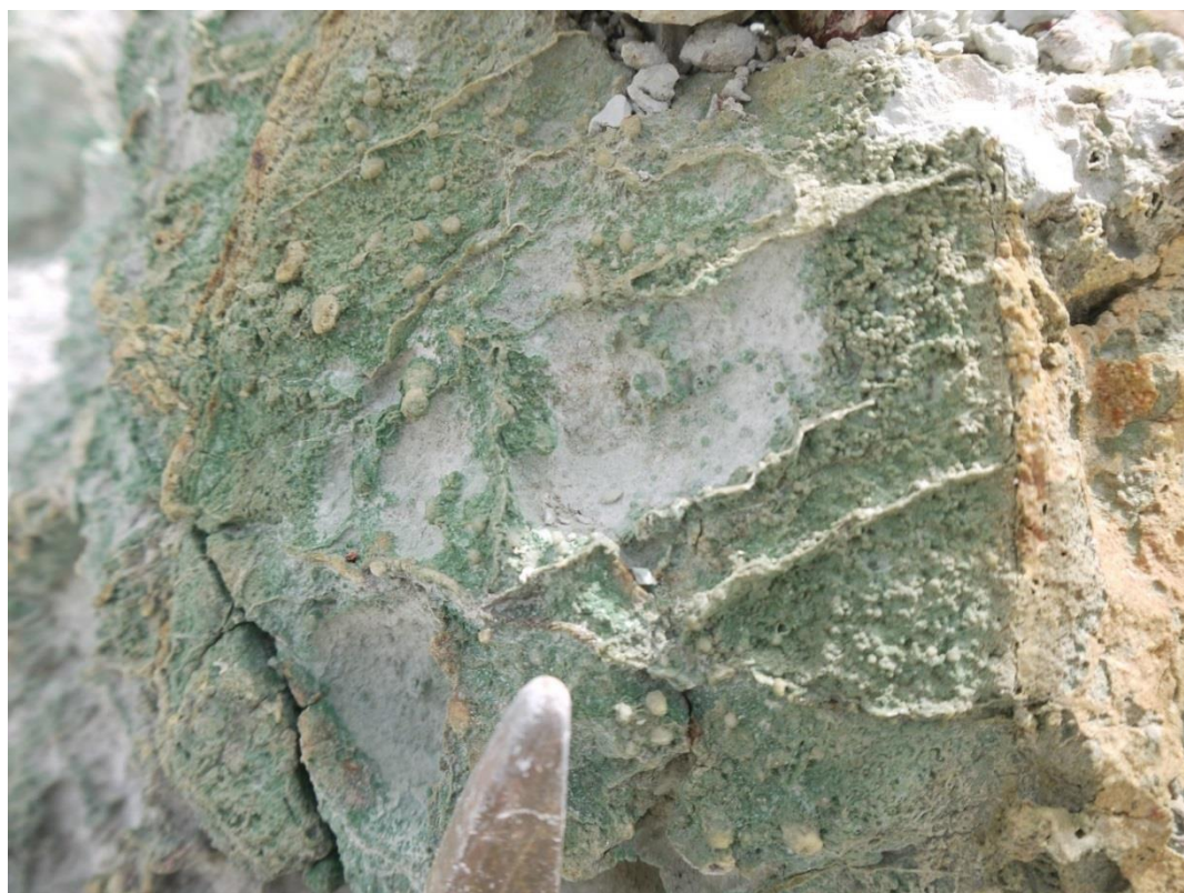
Figure A3.80: Quartz stringers with a chloritized quartz amygdaloidal basalt. Very common in almost all wall rock.
