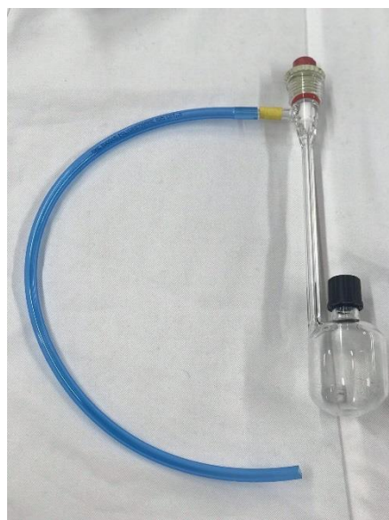
Figure 2.1. Catalyst testing using a Colaver reactor.
