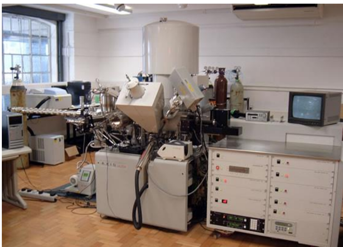
Figure 2.4. The Kratos Axis Ultra DLD X-ray photoelectron spectrometer used in this study.
