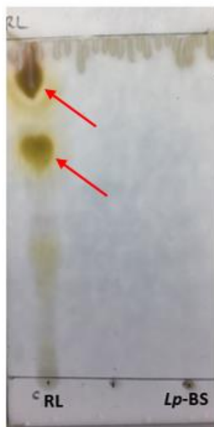
Figure 3.9 Thin layer chromatography of Lp -BS . The extracted biosurfactant Lp -BS demonstrated no lipid spot following staining with ammonium molybdate/cerium IV sulphate stain while the two lipid moieties of the mono- and di-rhamnolipid (RL) positive control are shown as brown spots (red arrows).
