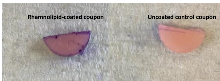
Figure 4.5 Crystal violet staining of acrylic discs coated with rhamnolipid 50 mg/mL. Crystal violet binds to the mannose moiety of the rhamnolipid molecules. Therefore rhamnolipid coating can be detected with crystal violet. The image is a representative of three independent repeats.
