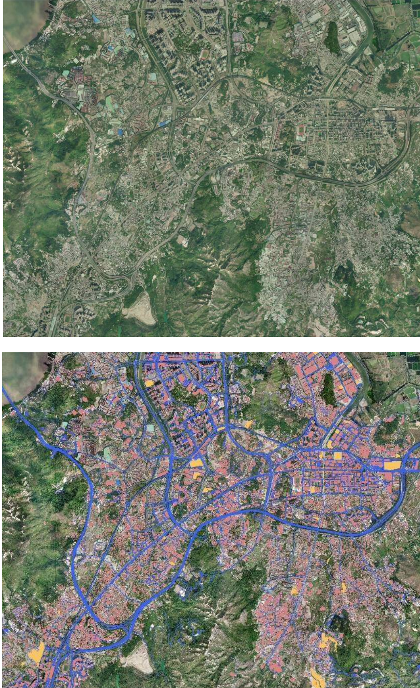
Figure C4. 9 Example of Overlaying the GIS data. (Top) Digital Orthophoto DOP5000 Map, (Bottom) Digital Orthophoto DOP5000 overlaid with the (1) Building, (2) Road, (3) Construction and (4) Sea data.
