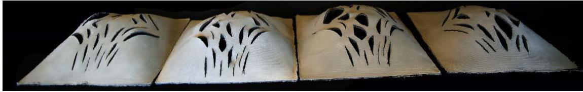
Figure 10: Concrete pieces from the training data set. The initial pattern is the same for all, the plunging and hydrating coordinates are randomly generated for each of them.
