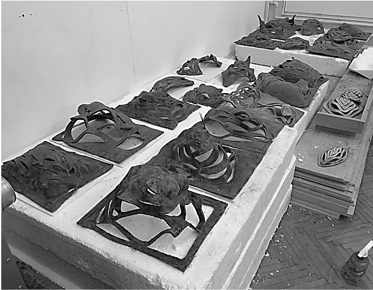
Figure 8: Catalogue of concrete shells resultant from all 25 participants. The boundary condition was the same for all. The pop-up pattern was designed and decided by each participant as well as the deformation during the process. Participants could go outside of the simulated shape
