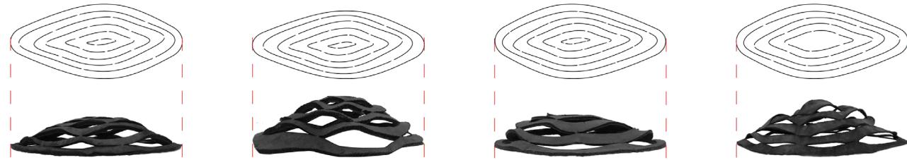
Figure 6: Comparison of geometric differences in the 3D pop-up surfaces; product of changes in boundary conditions and cutting patterns.
