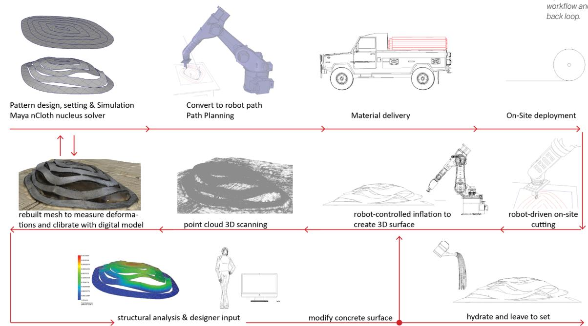
Figure 9: Path planning workflow and feedback loop.
