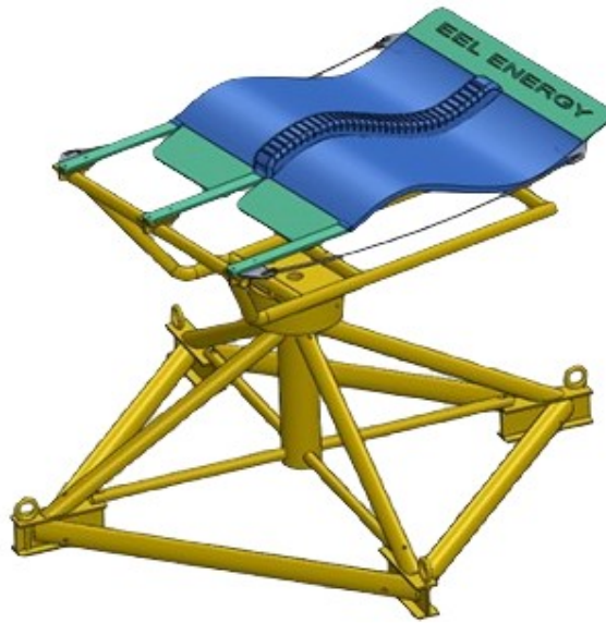
Figure 2.3: The EEL undulating membrane concept[36].
