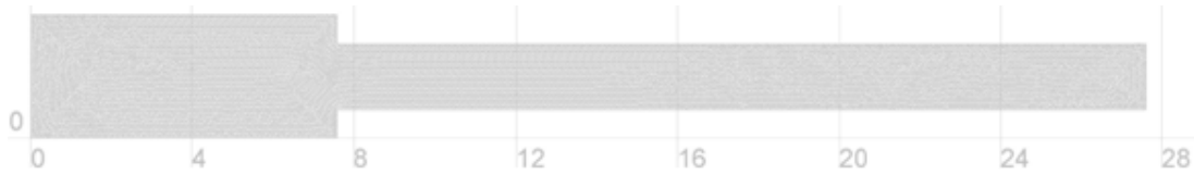
Figure 4.33: Computational mesh of flume, reduced in length to weir boundary. Dimensions given in m
