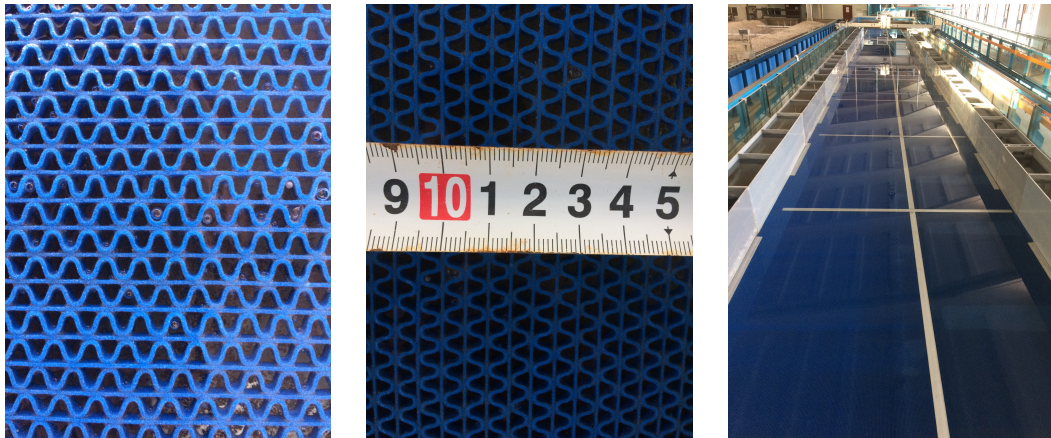
Figure 4.4: Rubber matting placed on the bed of the flume to increase bed roughness
