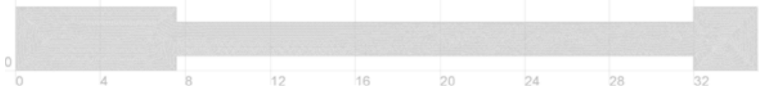
Figure 4.32: Computational mesh of flume for sluice gate control. Dimensions given in m
