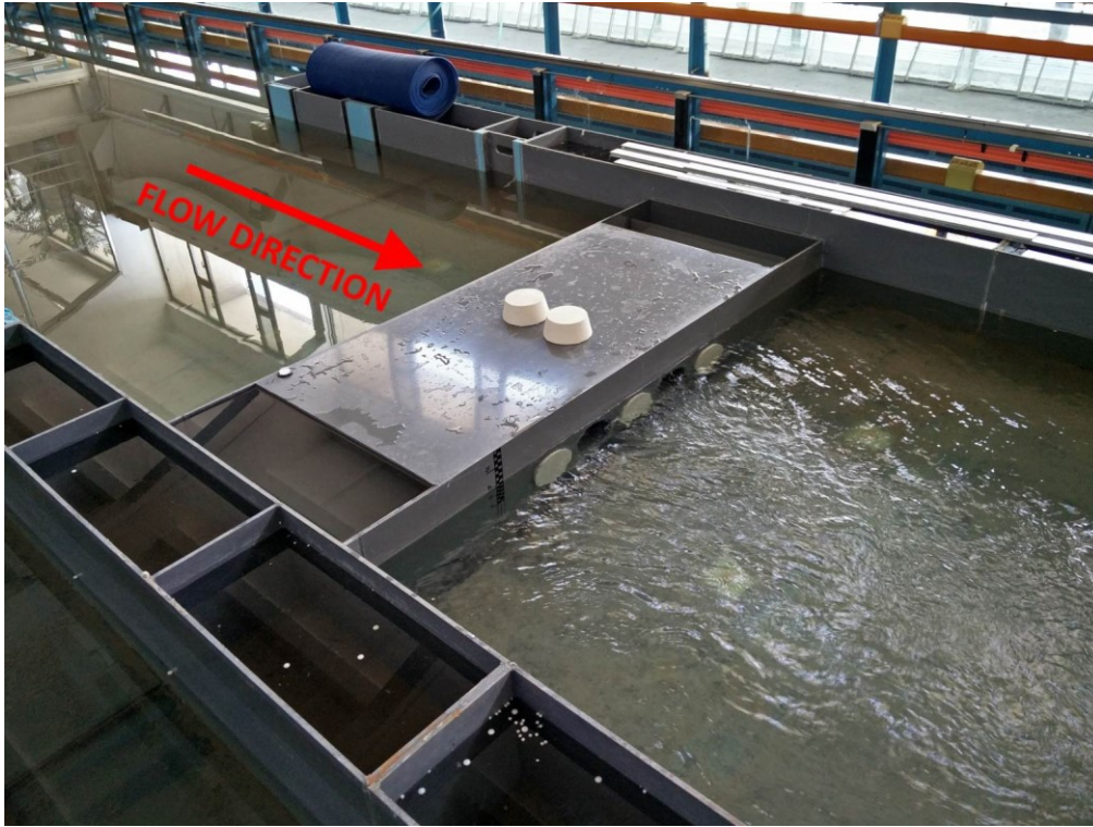
C.7: Running the experiment with two inner ducts open.
