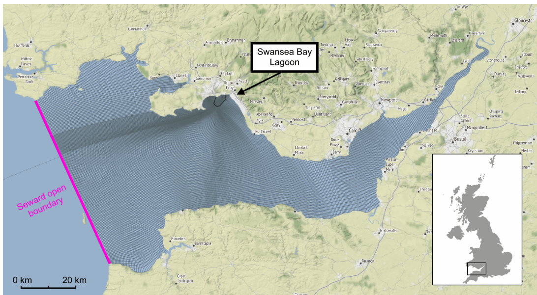
Figure 7.4: Domain of the model, overlaid with the computational grid.
