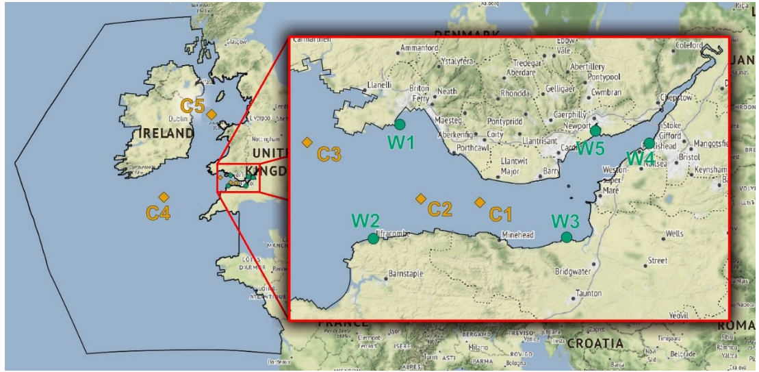
Figure 5.5: Locations of the observation sites used for validation of the tidal flow (yellow) and water levels (green).
