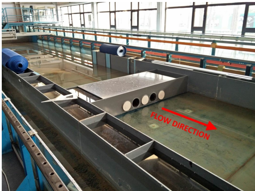
C.6: White silicone plugs were used to change the configuration of the open ducts.
