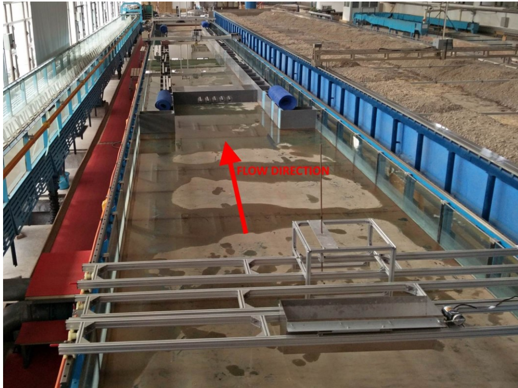
C.1: Bird's-eye view of an empty flume with the barrage already installed.
