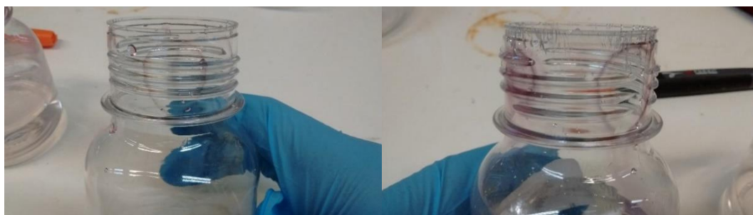
Figure 4-11: Photographs of a vial after the nebulisation of a gold suspension using the ATM-226 showing gold plating onto the walls acting as an impactor
