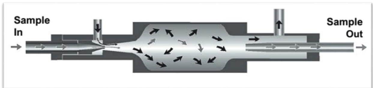
Figure 3-6: Diagram of the ICAO compliant Dekati DI-1000 ejector [19]
