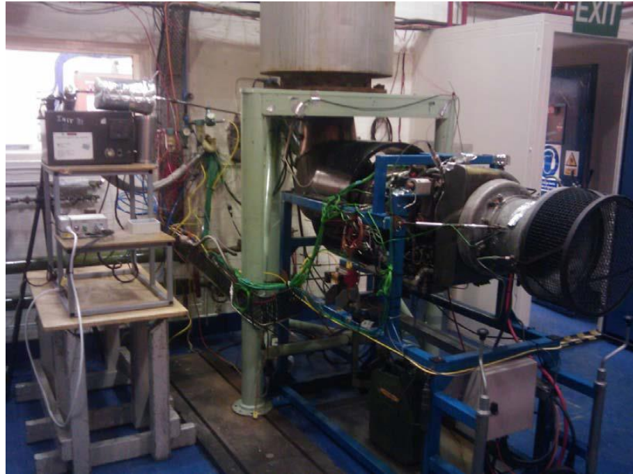
Figure 3-20: Photograph of a GNOME gas turbine rig with sample lines [19]
