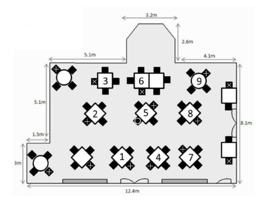
Figure 2.1 Aberdare Hall at Cardiff University where the BRIRs were recorded. Table layout and numbers are provided. The crosses represent locations of interferers and the circle is the KEMAR manikin location.
