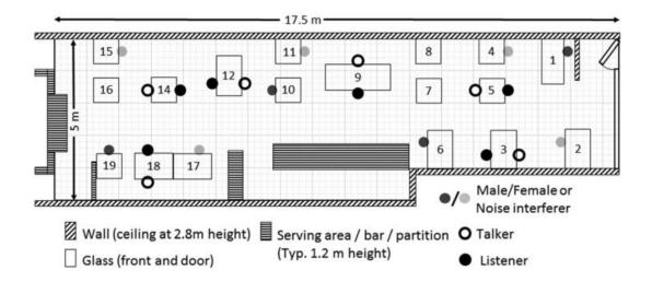
Figure 3.1 Plan view of Mezzaluna restaurant in Cardiff. Numbers in a box refer to table number. Black filled circles represent listener positions and the open circles are those of target talkers. Light grey circles are female interferers and darker grey are male interferers
