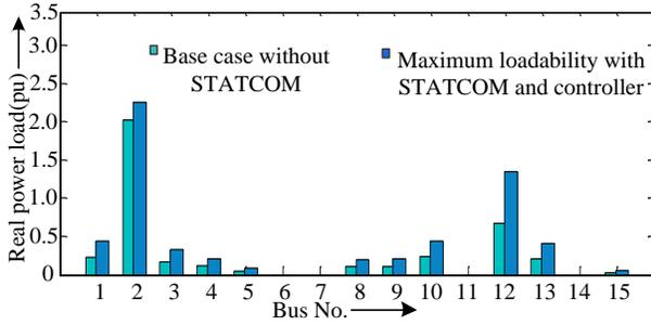
Figure 12: Load levels with and without STATCOM.
