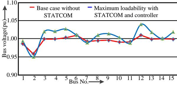
Figure 14: Voltage levels with and without STATCOM.
