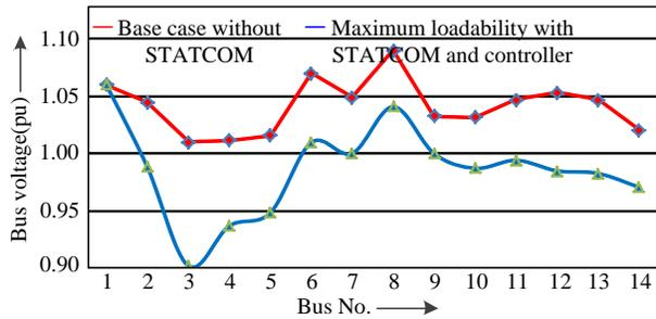
Figure 7: Voltage levels with and without STATCOM.
