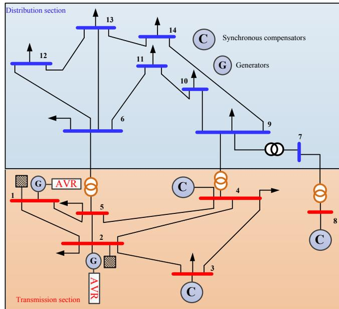
Figure 4: IEEE 14 bus test system
