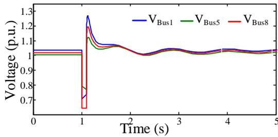
Figure 20: Voltages profile with SC at bus no. 1.
