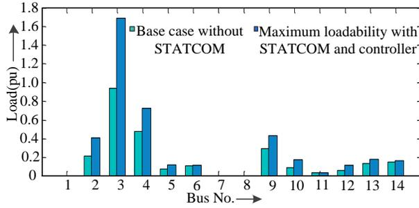
Figure 5: Load levels with and without STATCOM
