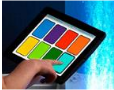
Figure 4.1. Photograph of the iPad 2 running the S4 app displaying of all eight buttons that can be used to change the colours on certain pieces of equipment (see Table 4.2).
