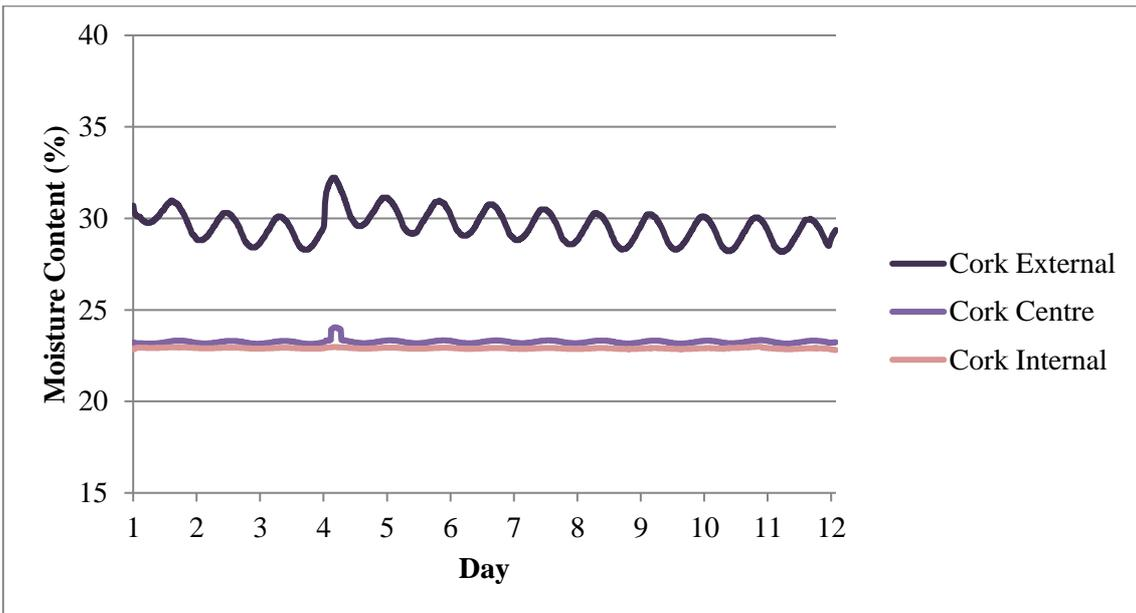
Figure 15. Interstitial moisture content (%) measured in Cork panel from 02/10/2017 to 13/10/2017 under dynamic conditions.
