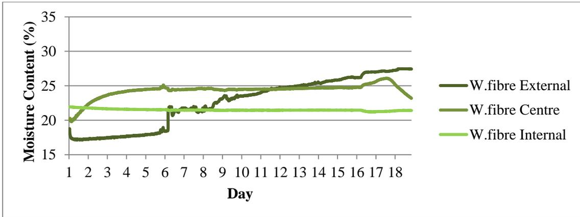
Figure 13. Interstitial moisture content (%) measured in Woodfibre and Woodwool panel from 14/09/2017 to 02/10/2017 under steady state conditions.
