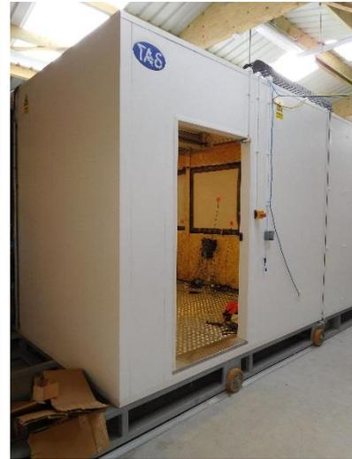
Figure 8. Dual climate chamber
