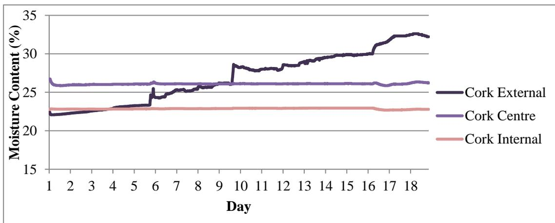
Figure 12. Interstitial moisture content (%) measured in expanded Cork panel from 14/09/2017 to 02/10/2017 under steady state conditions.
