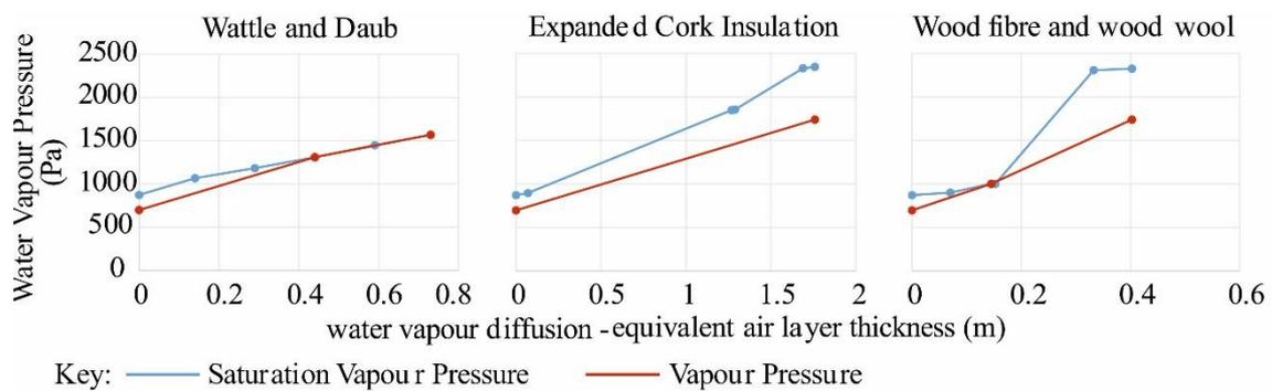
Figure 9. Glazer calculations according to BS EN ISO 13788:2012 for three infill panel constructions with external (left) conditions of 5°C and 80% RH and internal (right) conditions of 21°C and 70% RH. Source: (Author's own, 2017)
