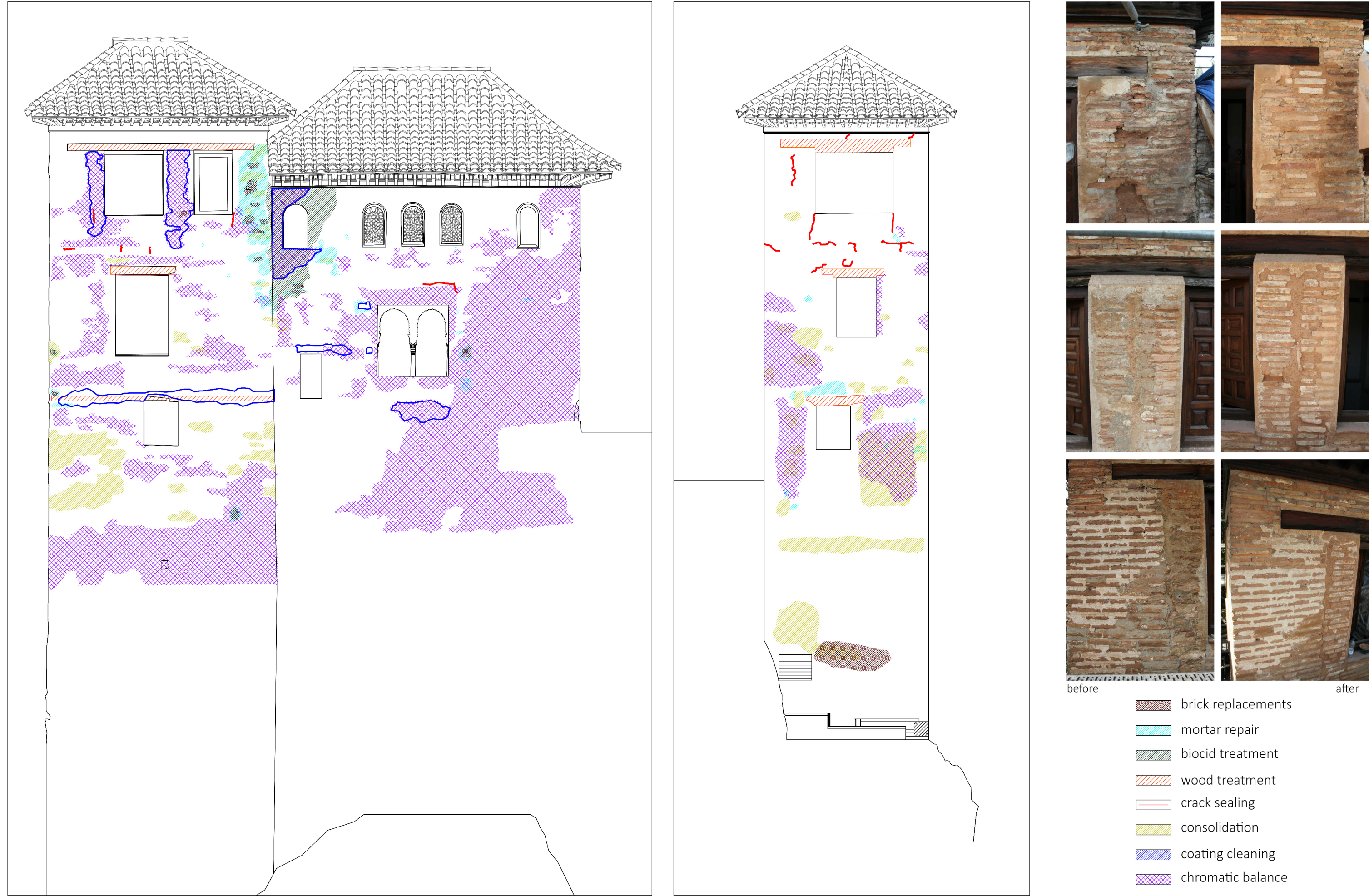
Fig.38 Interventions of the external brickwork walls. North-east and south-east elevations
