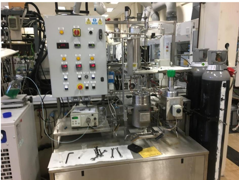
**Figure 2.2: Photograph of the Separex build supercritical rig set up for the SAS method used to make the oxide in this thesis**
