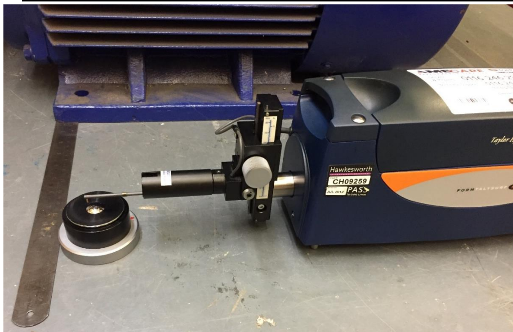
Figure 5.8 Talysurf calibration using calibration ball on the floor.
