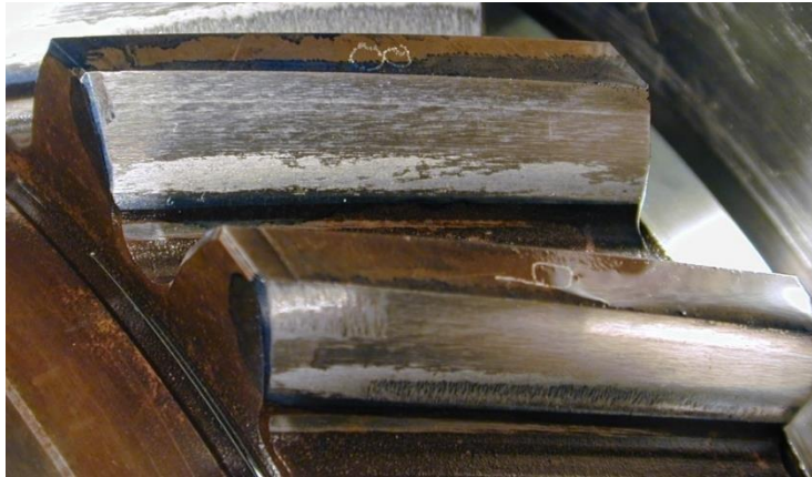
Figure 1.9 Micropitting predominantly in the dedendum region of a helical test gear tooth.
