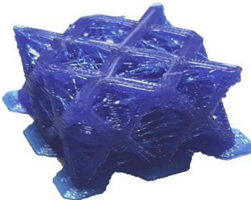
Figure A.3: Octet-truss geometry printed at Cardiff University using ninjaflex.
