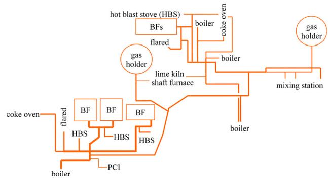
Fig. 3. The physical model of a BFG sub-network.
