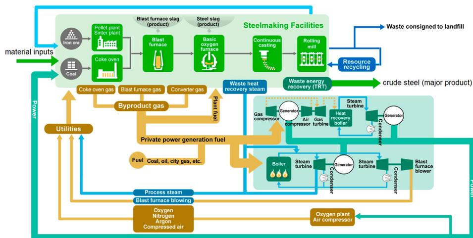
Fig. 2. Material and energy flows in BF–BOF steelworks [25].
