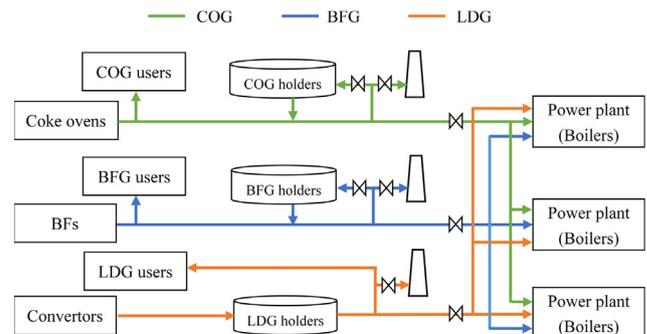
Fig. 4. The physical model of a gas network [72].
