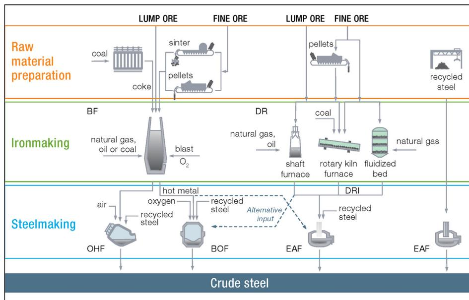
Fig. 1. Iron and steel production routes [14].
