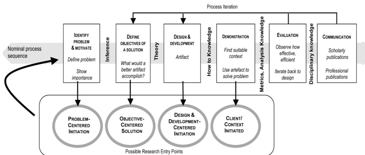
Figure 15 Design Science Research Methodology (DSRM) Process Model (Peffers et al., 2007)
