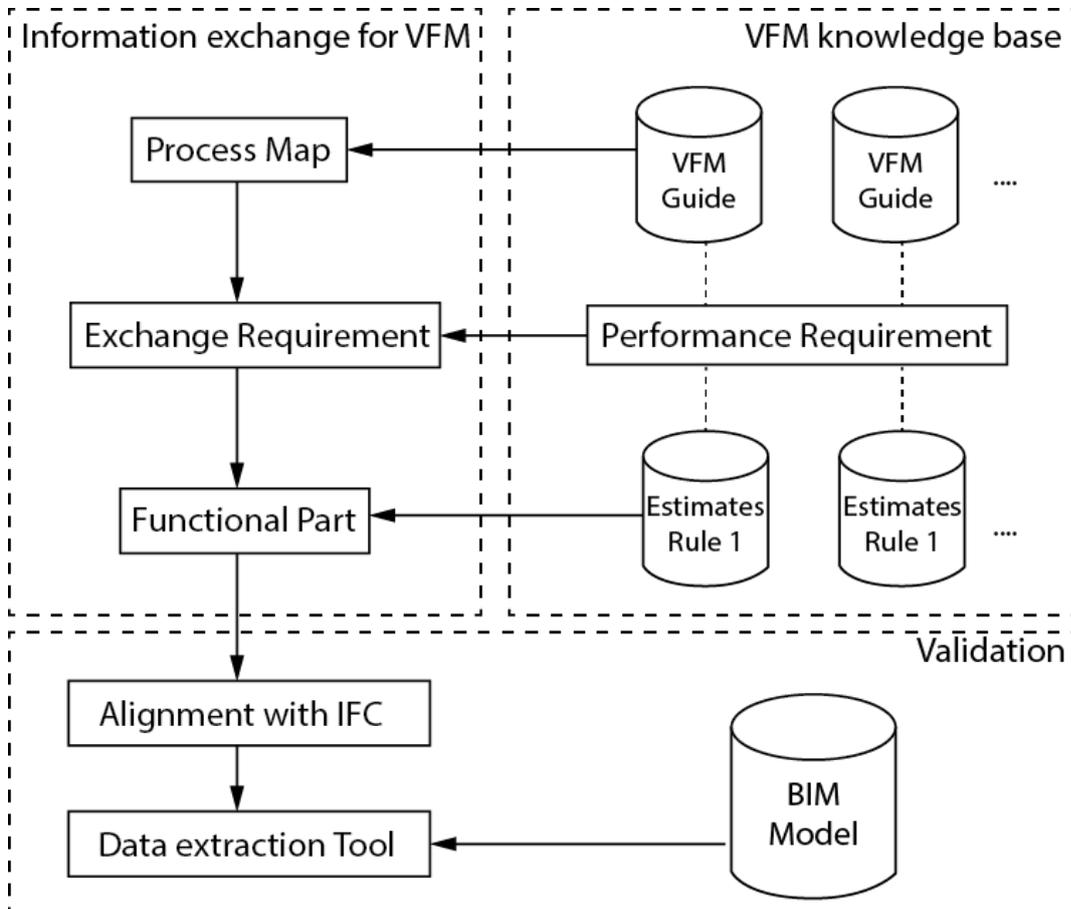
Figure 17 Framework for implementing Vfm information exchange scheme using BIM
