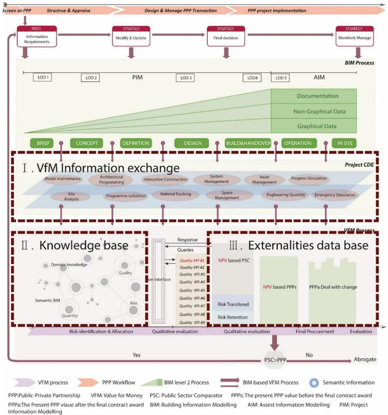
Figure 59 Proposed BIM-based VfM roadmap align with the current standardized BIM process.
