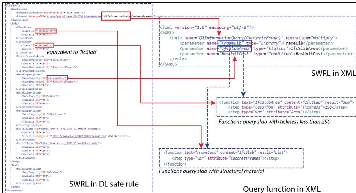
Figure 52 The integrated connections between SWRL and query functions
