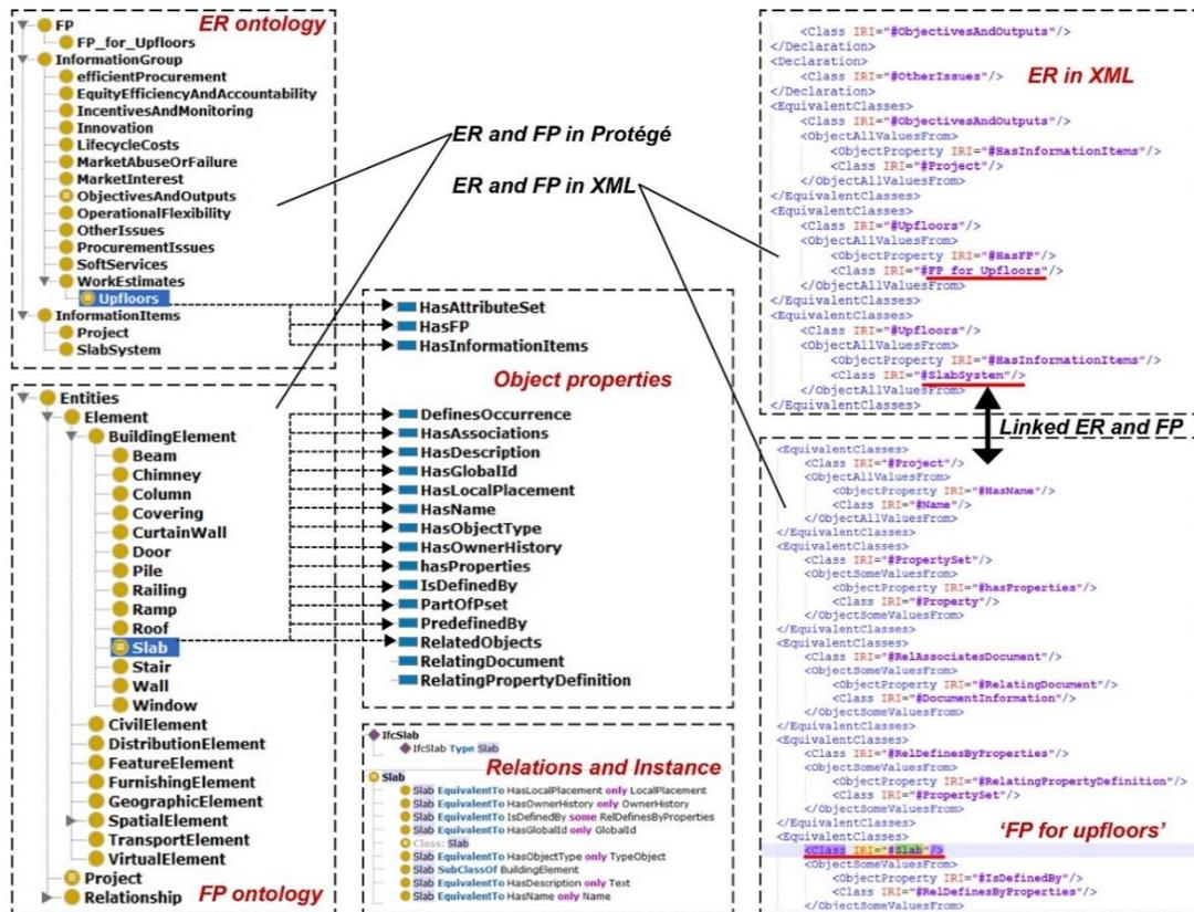
Figure 24 VIM exchanges in Protégé and OWL/XML
