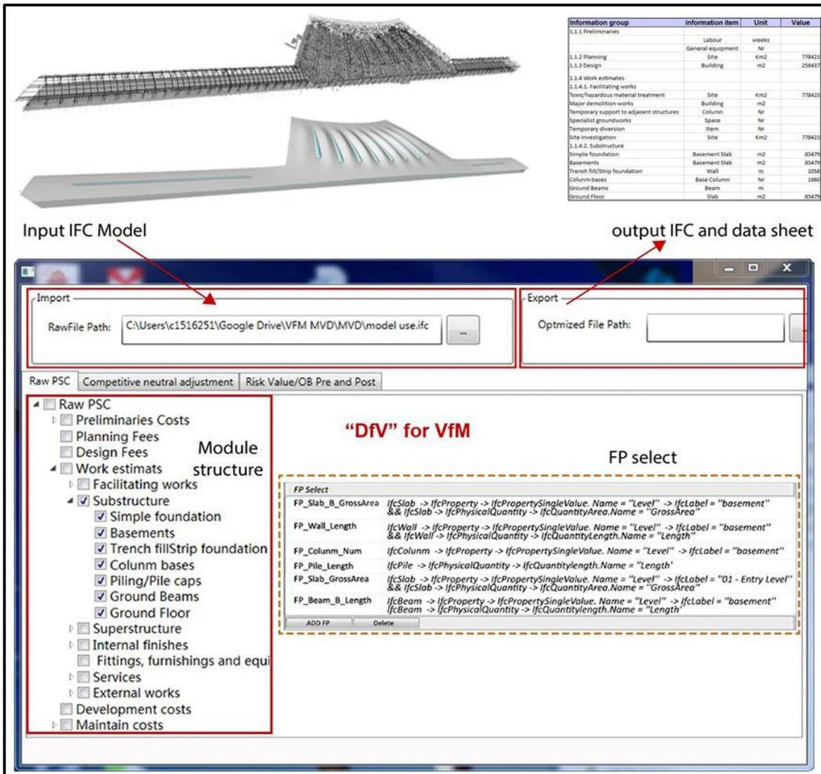
Figure 28 DfV interface and data extraction process on airport BIM mode
