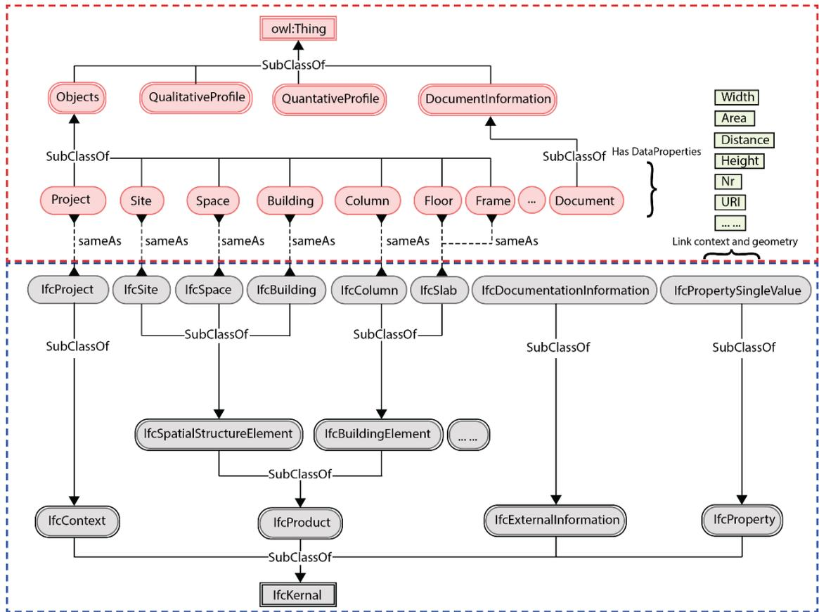
Figure 47 Alignment of classes between the VfMO and IfcOwl.
