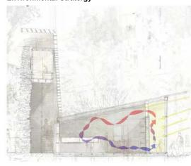
The classrooms are designed with a passive environmental strategy to maximise environmental gains. The classrooms are heavily insulated with a large stone wall at the rear of the building with a high thermal mass.
