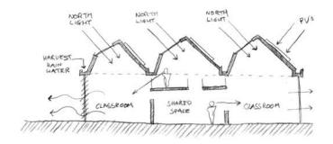
The whole structure is designed around the simple shapes of geometry. The classrooms are planned on a square grid and the bracing within the roof structure is based on the types of triangle.
