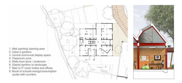
Figure 101: Class 2 plan and inhabited section
