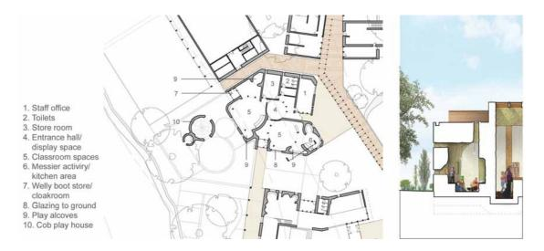
Figure 98: Reception class plan and inhabited section
