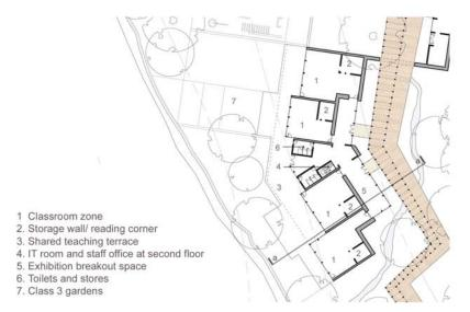
**Building form:** Class 3 follows the contours of the land, with a maintained internal ceiling height, the interlocking pitched roofs of the classrooms echoes the rows of terraced housing on the valley slopes.
