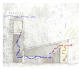
In warmer months the porch acts as a buffer to the sun allowing the classroom to be cooled through natural stack ventilation behind. The classrooms harvest rainwater from their roofs for use in toilets and on the allotments. The geography and conditions of the valley site are conducive for the production of renewable wind energy. The bell towers which give legibility to the site also act as a ventilating chimney to the classroom and means of energy production via the wind turbine at their top.
