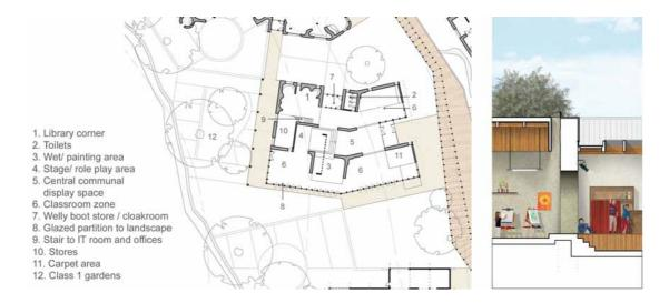
Figure 99: Class 1 plan and inhabited section
