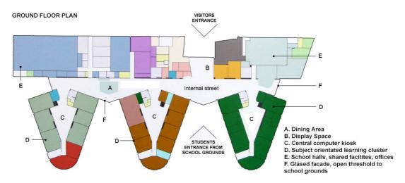
Figure 18: Ground floor plan of the Bristol Metropolitan
