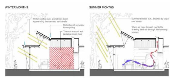
Figure 105: Passive lighting/ventilation strategy for class 1\_ highlighting typical considerations for teaching spaces
