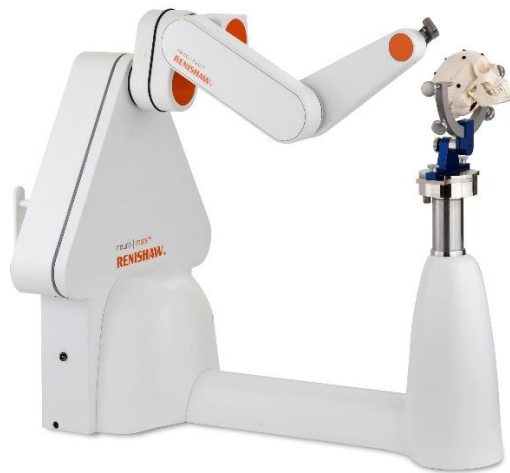
Figure 2 – The ‘neuromate™’ surgical robot utilises multiple degrees of freedom to attain the precise insertion location and trajectory as determined in the surgical plan. Adapted from promotional material (3).
