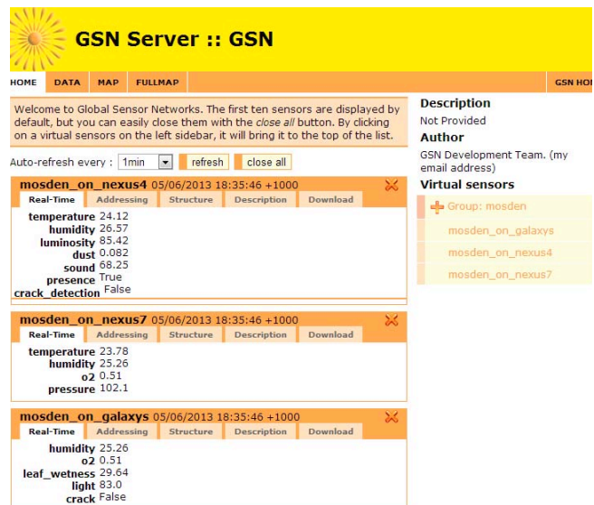
Fig. 6: Screenshot of a cloud GSN instance showing three different MOSDEN instances registration
