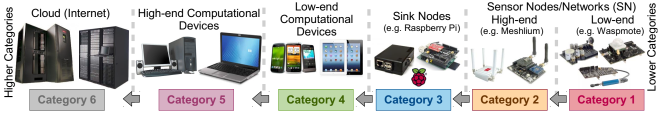
Fig. 1: Categorization of IoT devices based on their computational capabilities. The devices belong to each category has different capabilities depending in term of processing, memory, and communication. They are also different in price where devices becomes more expensive when move to left. The computational capabilities are also get increased when move to left.
