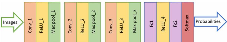
**Fig. 5** Schematic architectures of the CIFAR classification network
