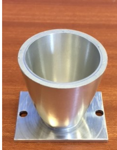
Figure 3.20: CPC design manufactured by a CNC machine.
