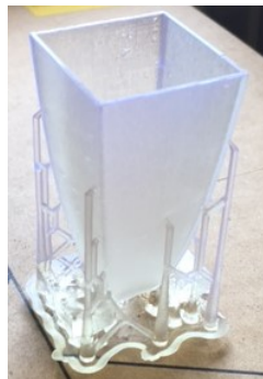
Figure 3.18: 3D printed CCPC with supports using Form +1.
