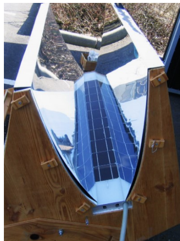
Figure 2.20: Symmetric CPC reflector with 10-cell module string [94].
