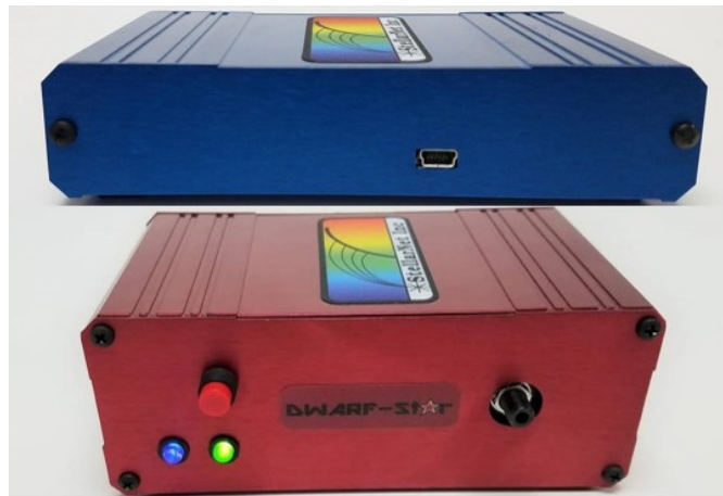
Figure 3.10: A photograph of the blue (UV-VIS) and red (IR) instruments for measuring sunlight spectrum over a range of 200 nm to 1700 nm.
