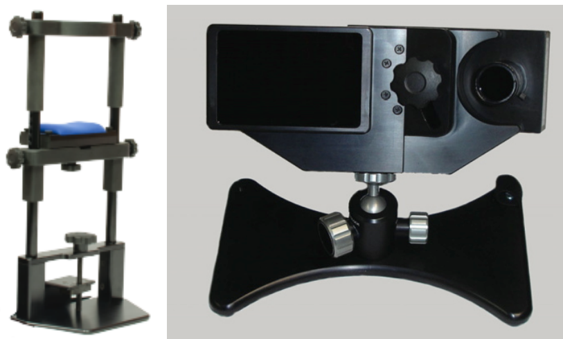
Figure 5 - EyeLink 1000+ head mount and EyeLink 1000+ in desktop configuration
