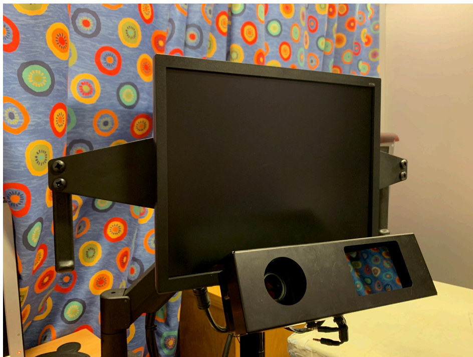
Figure 38 - EyeLink 1000 in the arm mount configuration
