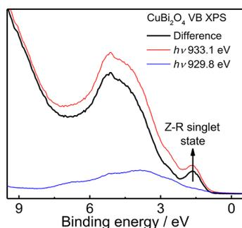
**Figure 2.** Valence band photoemission of  $\text{CuBi}_2\text{O}_4$  near the Fermi level showing the spectral intensity difference between on-resonance (at  $h\nu = 933.1$  eV) and off-resonance (at  $h\nu = 929.8$  eV) spectra.
