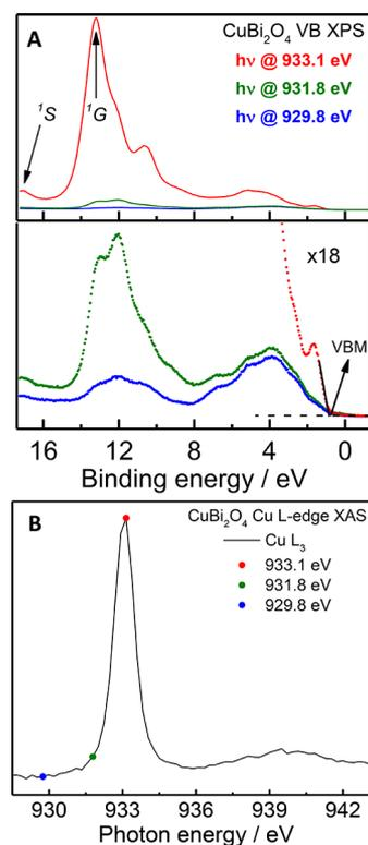
**Figure 1.** (A) Valence band photoemission spectra of  $\text{CuBi}_2\text{O}_4$  taken using photon energies near the Cu  $L_3$ . (B) Cu  $L_3$  X-ray absorption spectrum of  $\text{CuBi}_2\text{O}_4$  indicating the selected photon energies for the resonant photoemission experiment.
