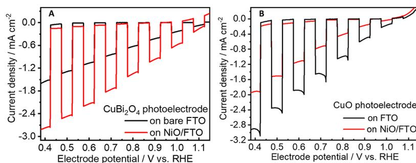
**Figure 6.** (A) Chopped-light linear sweep voltammetry scans for CuBi<sub>2</sub>O<sub>4</sub> (black) and NiO/CuBi<sub>2</sub>O<sub>4</sub> (red) photoelectrodes. (B) Chopped-light linear sweep voltammetry scans for CuO (black) and NiO/CuO (red) photoelectrodes. PEC measurements were done in 0.2 M K<sub>2</sub>SO<sub>4</sub> + 0.1 M phosphate buffer solution (pH 6.8) with 0.3% w/w H<sub>2</sub>O<sub>2</sub>.
