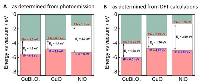
**Figure 5.** (A) Measured and (B) calculated electron affinity (CBM) and ionization potential (VBM) of CuBi<sub>2</sub>O<sub>4</sub>, CuO, and NiO with respect to the vacuum level.
