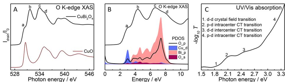
**Figure 4.** (A) O K-edge XAS of CuBi<sub>2</sub>O<sub>4</sub> along with that of CuO for comparison. (B) Empty PDOS from DFT calculations for CuBi<sub>2</sub>O<sub>4</sub>; the O K-edge XAS is included in the same scale for comparison. (C) UV-vis absorption spectrum of CuBi<sub>2</sub>O<sub>4</sub>.
