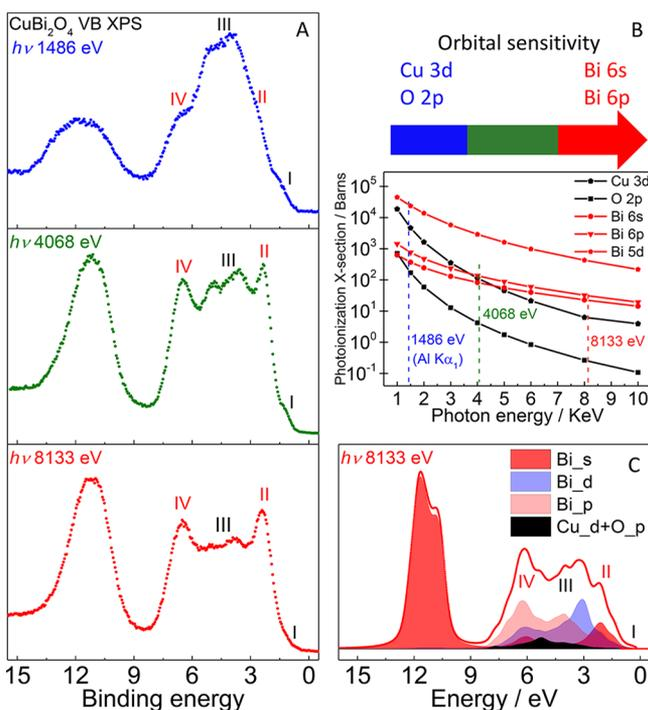
**Figure 3.** (A) Experimental VB photoemission spectra of  $\text{CuBi}_2\text{O}_4$  measured with 1486 eV ( $\text{Al K}\alpha_1$ ), 4068 eV, and 8133 eV ionizing photon energy. (B) Photoionization cross section dependence on the ionizing photon energy for valence orbitals in  $\text{CuBi}_2\text{O}_4$ .<sup>27</sup> (C) Calculated VB photoemission spectra of  $\text{CuBi}_2\text{O}_4$  at 8133 eV ionizing photon energy.
