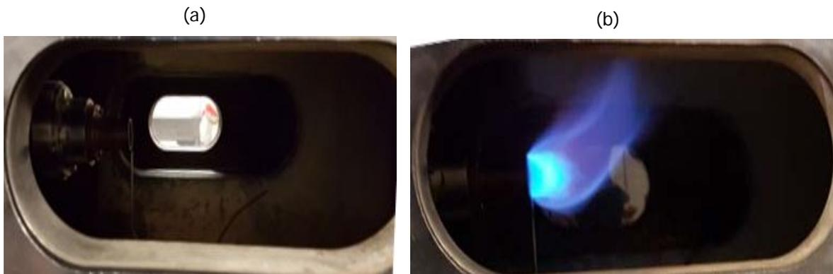
Figure 5-1: 25 mm Bunsen burner horizontal set-up, as installed (a) and with CH<sub>4</sub>-air flame (b)
