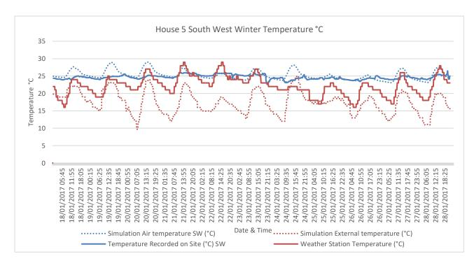
Figure 7.23 House 5 Simulation Temperature Comparison Winter – SW
