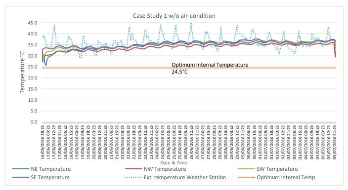
Figure 4.1- Internal temperature compared to external temperature- Case Study 1
