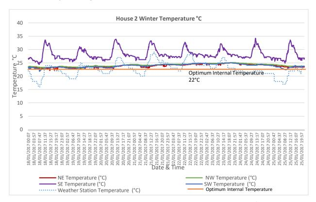
Figure 4.29- Internal temperature compared to external temperature- Case Study 2 without A/C
