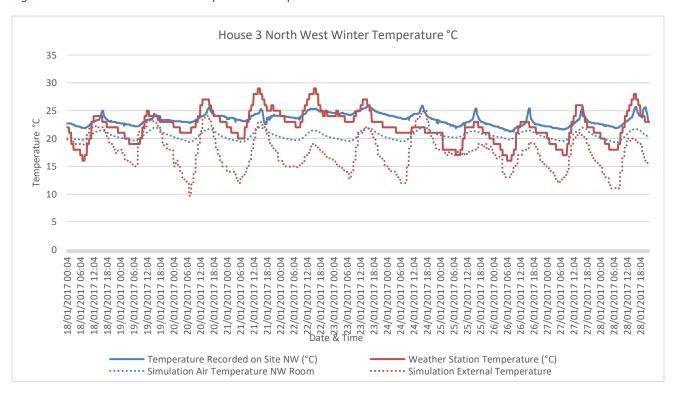
Figure 7.14 - House 3 Simulation Temperature Comparison Winter - NW
