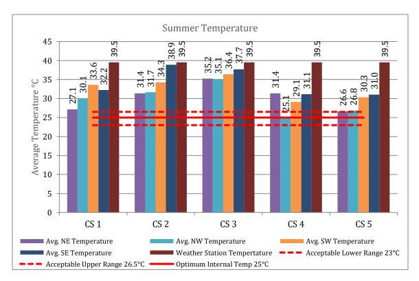
Figure 6.1- Comparison of Average Internal Temperature of Case Studies (CS) in Summer
