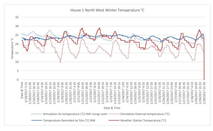
Figure 7.8 House 1 Simulation Temperature Comparison Winter – NW
