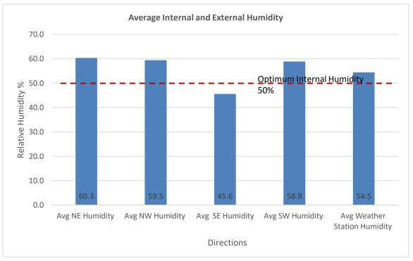
Figure 4.32- Average Internal and External Humidity - Case Study 2
