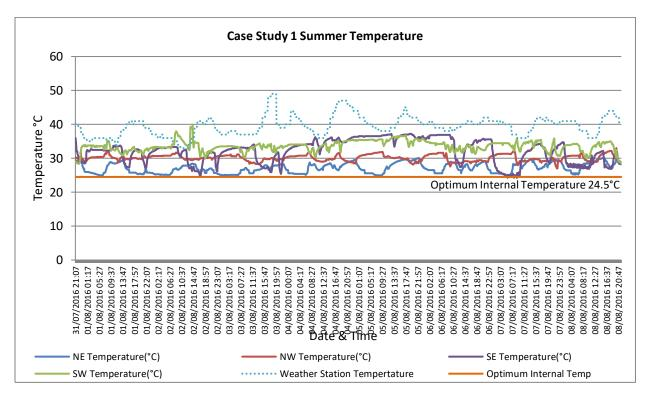
Figure 4.5- Internal temperature compared to external temperature- Case Study 1 with A/C
