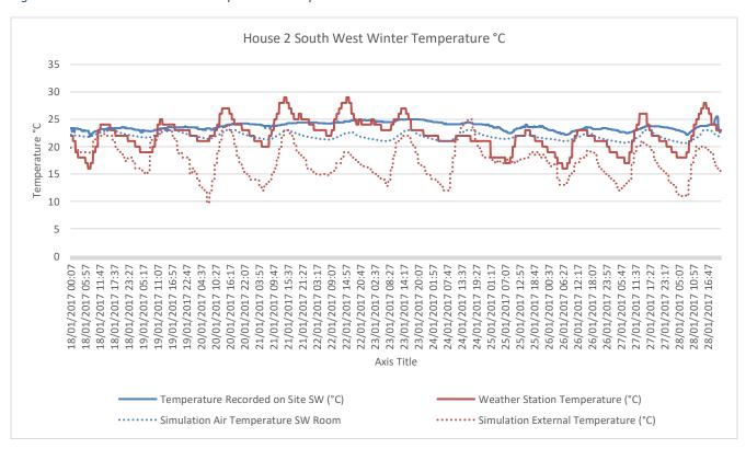
Figure 7.12 - House 2 Simulation Temperature Comparison Winter - SW
