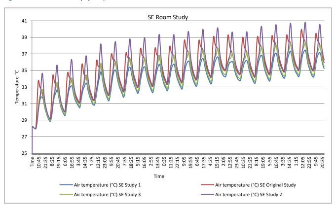
Figure 7.30- Simulation study of Temperature in SE Room
