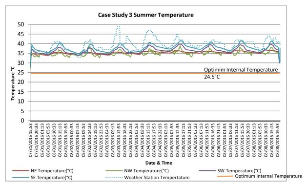
Figure 4.13- Internal temperature compared to external temperature- Case Study 3 with A/C
