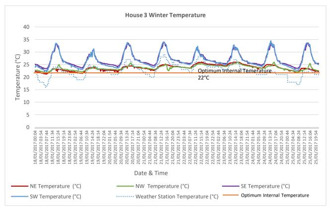
Figure 4.33- Internal temperature compared to external temperature- Case Study 3 without A/C
