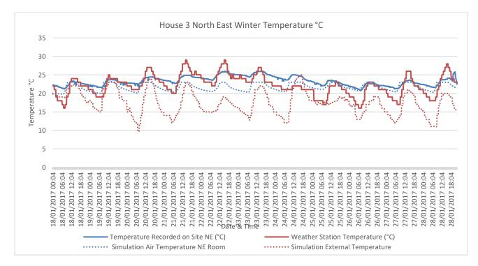
Figure 7.13 - House 3 Simulation Temperature Comparison Winter – NE
