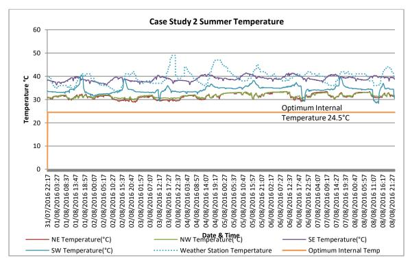
Figure 4.9 - Internal temperature compared to external temperature- Case Study 2 with A/C
