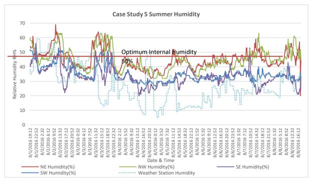
Figure 4.22 - Internal humidity compared to external humidity- Case Study 5 with A/C
