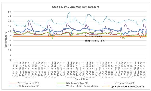
Figure 4.21- Internal temperature compared to external temperature- Case Study 5 with A/C
