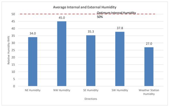
Figure 4.20 - Average Internal and External Humidity Case Study 4
