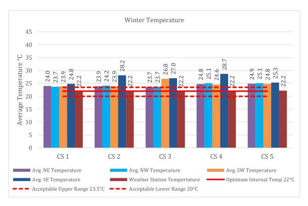
Figure 6.2- Comparison of Average Internal Temperature of Case Studies (CS) in Winter
