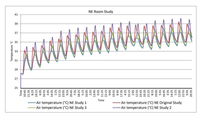
Figure 7.29 - Simulation study of Temperature in NE Room
