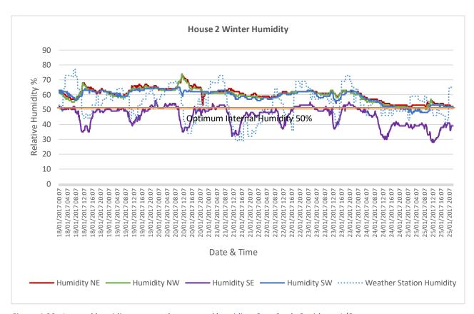
Figure 4.30 - Internal humidity compared to external humidity- Case Study 2 without A/C
