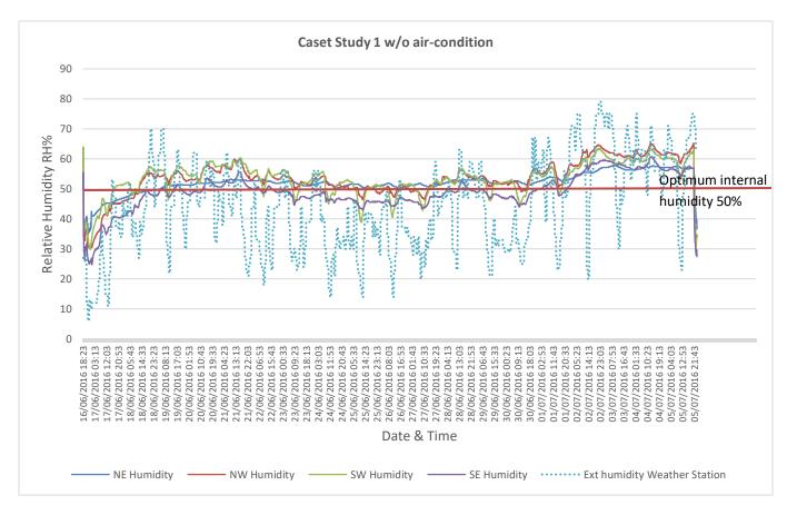
Figure 4.2 - Internal humidity compared to external humidity - Case Study 1
