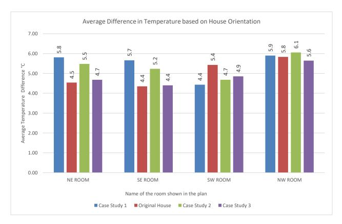
Figure 7.33 - Temperature Difference Compared to Weather Station Temperature
