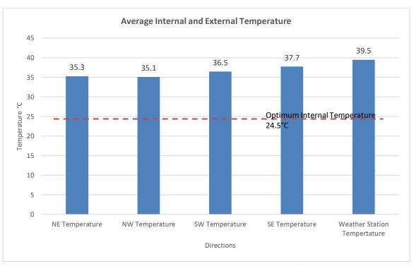
Figure 4.15 - Average internal and external temperature - Case Study 3 with A/C
