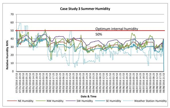
Figure 4.14 - Internal humidity compared to external humidity- Case Study 3 with A/C
