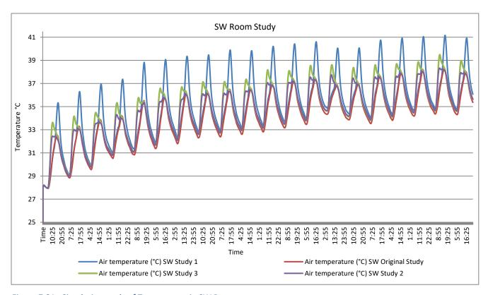
Figure 7.31 - Simulation study of Temperature in SW Room
