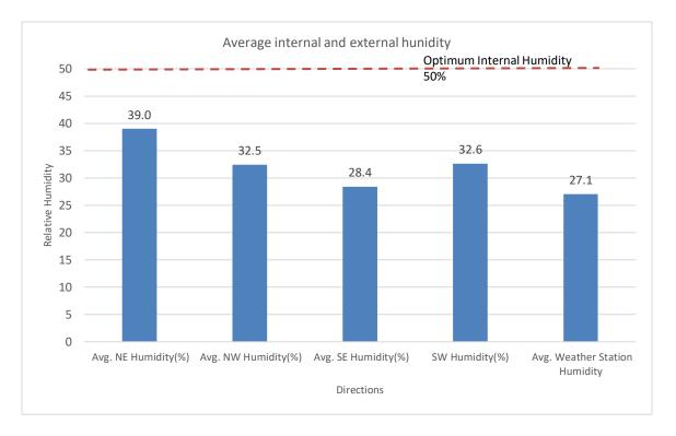
Figure 4.8- Average internal and external humidity - Case Study 1 with A/C
