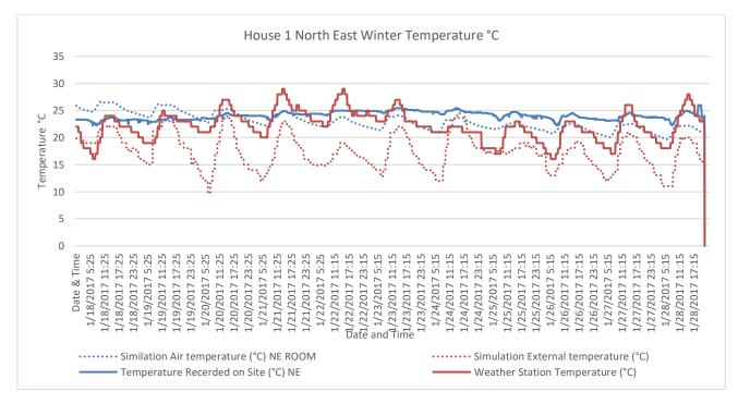
Figure 7.5 House 1 Simulation Temperature Comparison Winter – NE
