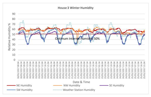
Figure 4.34 - Internal humidity compared to external humidity- Case Study 3 without A/C
