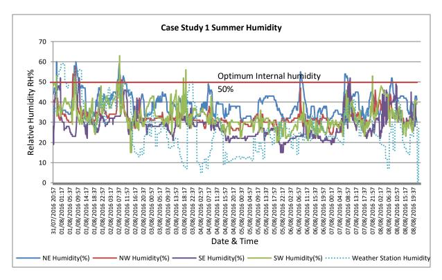
Figure 4.6 - Internal humidity compared to external humidity- Case Study 1 with A/C
