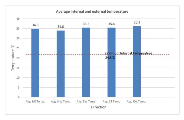
Figure 4.3 - Average internal and external temperature - Case Study 1
