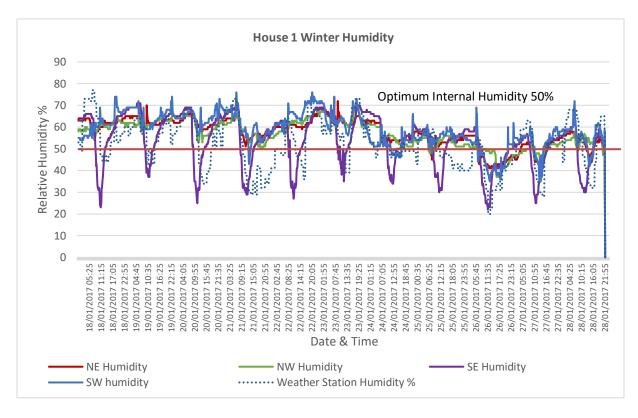
Figure 4.26- Internal humidity compared to external humidity- Case Study 1 without A/C
