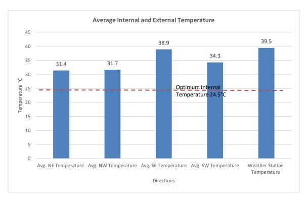
Figure 4.11- Average internal and external temperature - Case Study 2 with A/C
