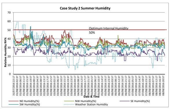
Figure 4.10- Internal humidity compared to external humidity- Case Study 2 with A/C
