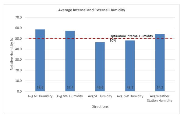
Figure 4.36 - Average Internal and External Humidity - Case Study 3
