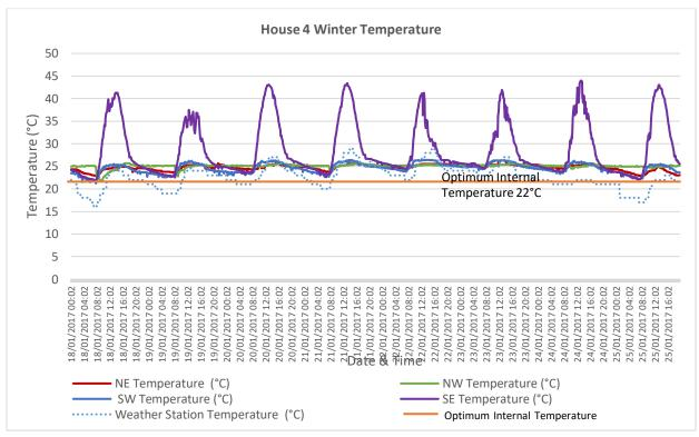
Figure 4.37- Internal temperature compared to external temperature- Case Study 4 without A/C
