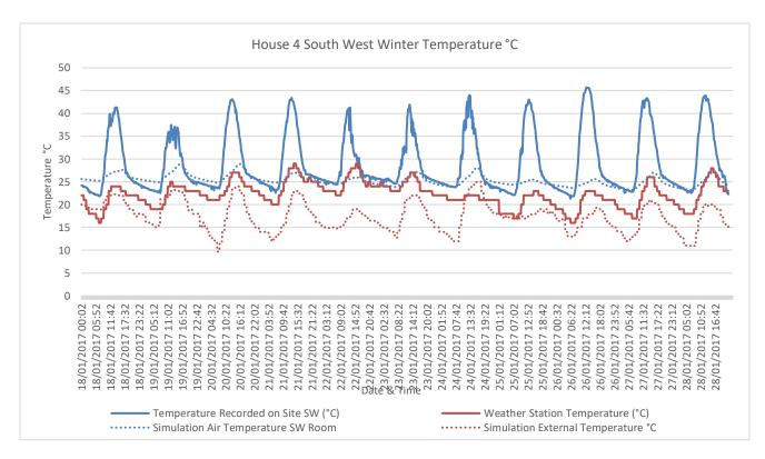
Figure 7.19 - House 4 Simulation Temperature Comparison Winter – SW
