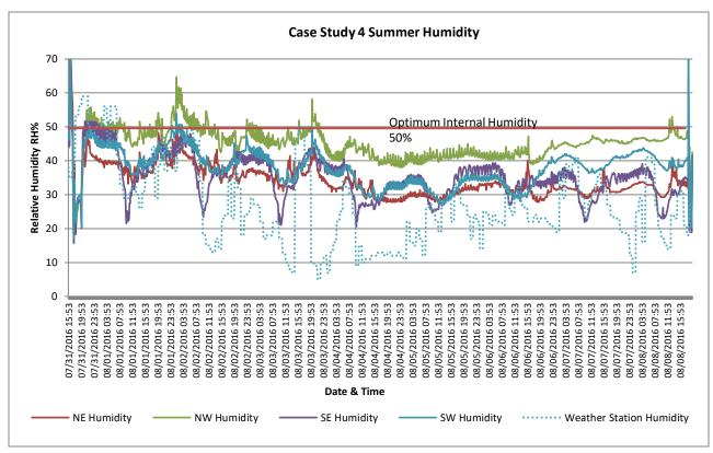
Figure 4.18 - Internal humidity compared to external humidity- Case Study 4 with A/C
