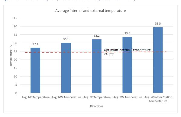
Figure 4.7- Average internal and external temperature - Case Study 1 with A/C
