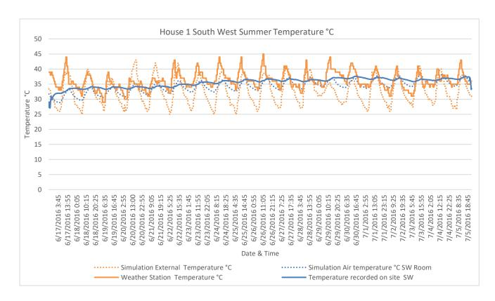
Figure 7.3 -House 1 Simulation Temperature Comparison – SW
