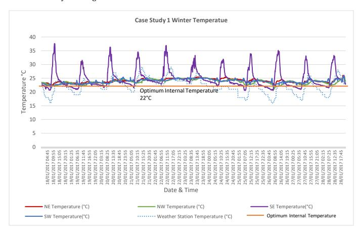
Figure 4.25 - Internal temperature compared to external temperature- Case Study 1 without A/C
