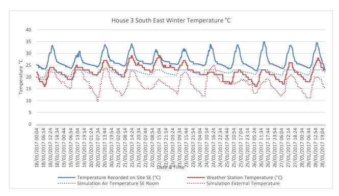
Figure 7.15 - House 3 Simulation Temperature Comparison Winter - SE
