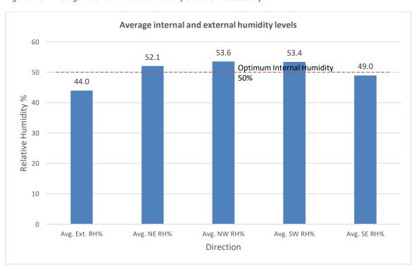
Figure 4.4- Average internal and external humidity levels - Case Study 1
