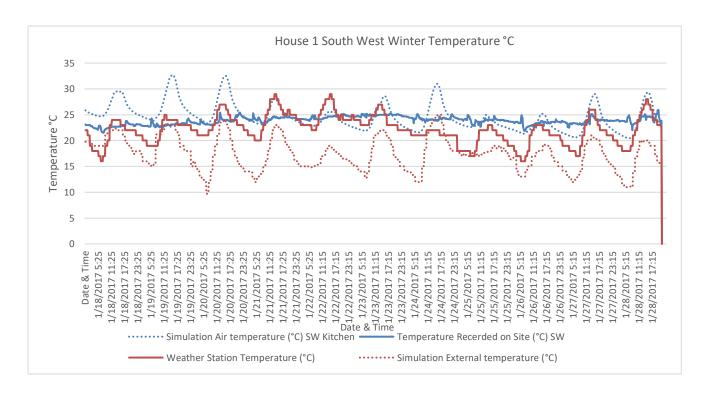
Figure 7.7 - House 1 Simulation Temperature Comparison Winter – SW
