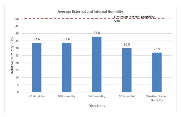
Figure 4.16 - Average internal and external humidity - Case Study 3 with A/C
