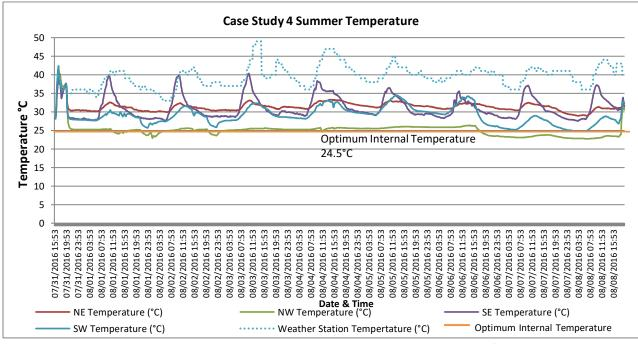
Figure 4.17- Internal temperature compared to external temperature- Case Study 4 with A/C
