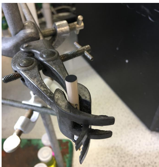
Figure 2.9. The prepared electrode of Au/C or Pd/C on glassy carbon electrode.
