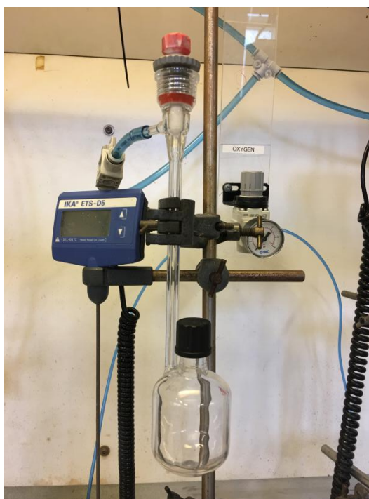
Figure 2.5. 50 mL colaver glass reactor, used in aqueous HMF, glycerol and ethanol oxidation.
