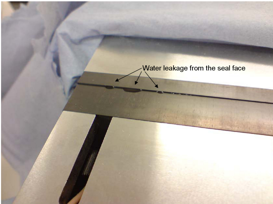
Figure 11. Water leakage from the graphite seal face at the end of Run 5.
