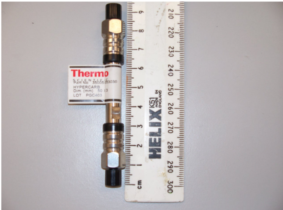
Figure 1. A Thermo Hypercarb HPLC column with a 50mm x 3mm active column and 5 \mu m particle size.
