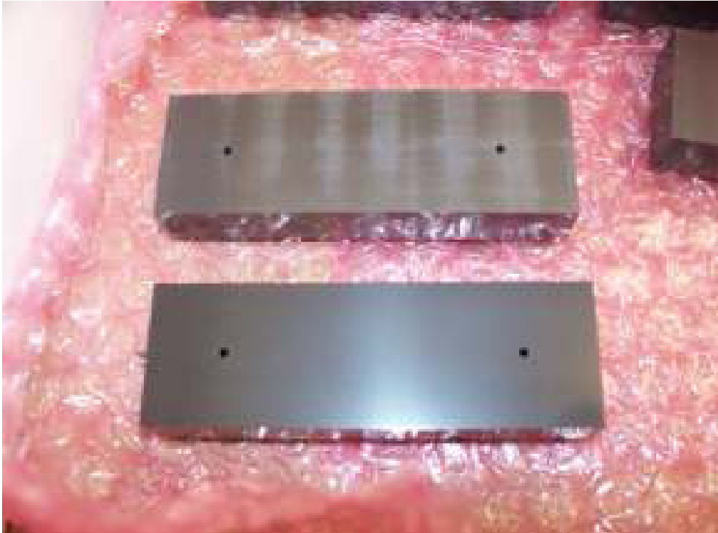
Figure 25. A visual comparison between the as supplied, ground finish graphite substrate and the polished graphite substrate.
