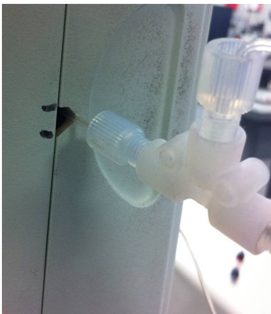
Figure 33. A close up of the cut-out machined into the Surveyor MSQ door to allow the tubing to directly interface to the ESI input.
