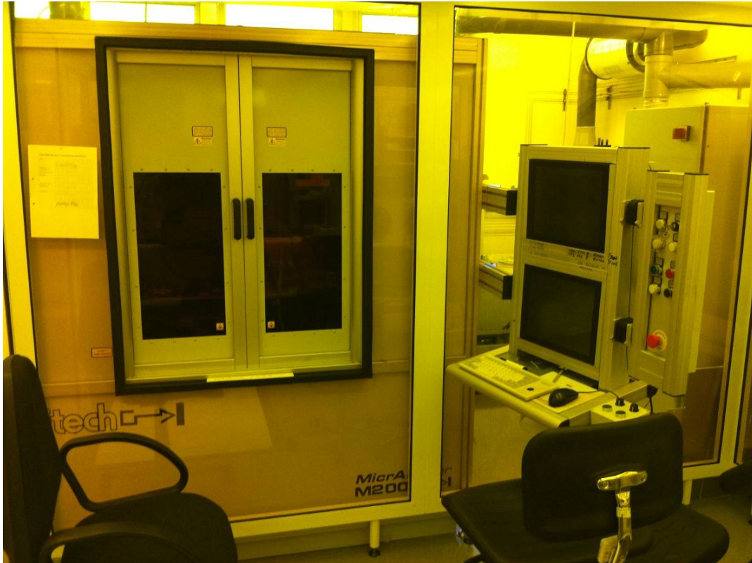
Figure 2. Front view of the Exitech M2000EF laser workstation showing operator console and load doors.
