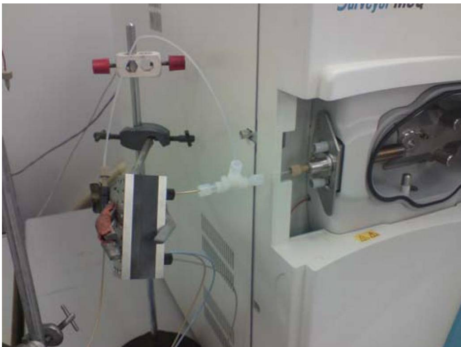
Figure 30. Assembled graphitic device interfaced with flow-make up to provide a sufficient volumetric flow for electrospray ionisation and mass spec analysis.
