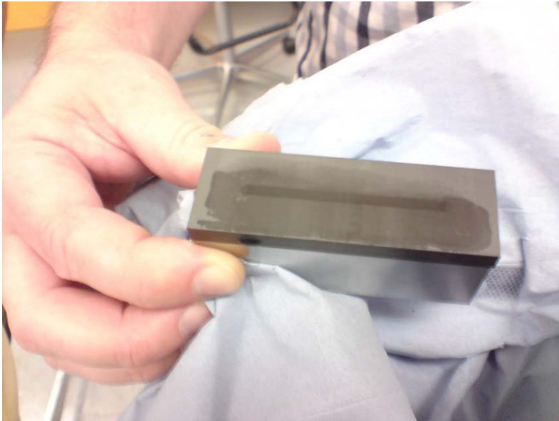
Figure 12. The water film on the graphite substrate surface after run 6.
