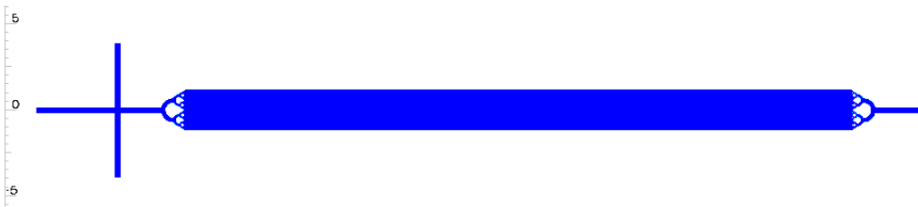
Figure 29. The complete CAD file used to write the separations column clearly showing the position of the X junction to the left. The CAD was written in Alphacam and AutoCAD and comprised of over 3200 component parts once translated into G-Code.
