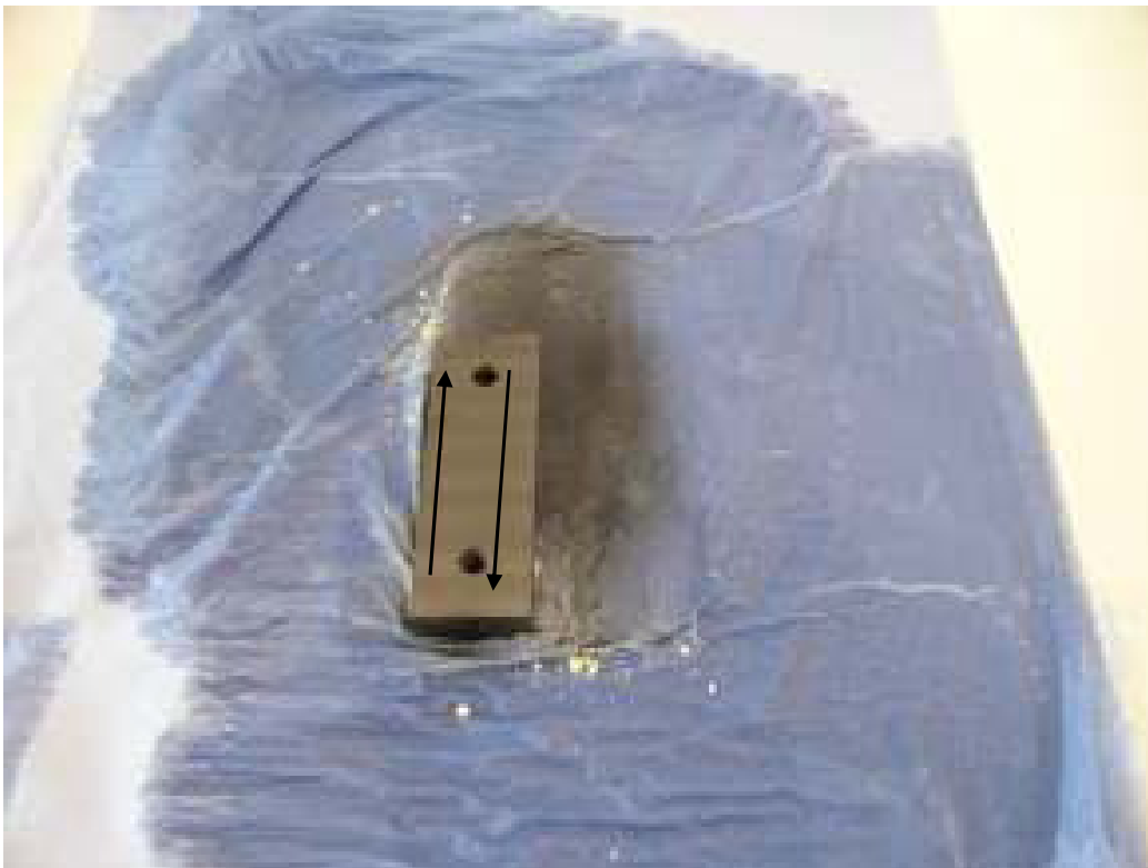
Figure 24. Polishing process, the arrows indicating the forward and backwards motion in the long-axis polishing direction.
