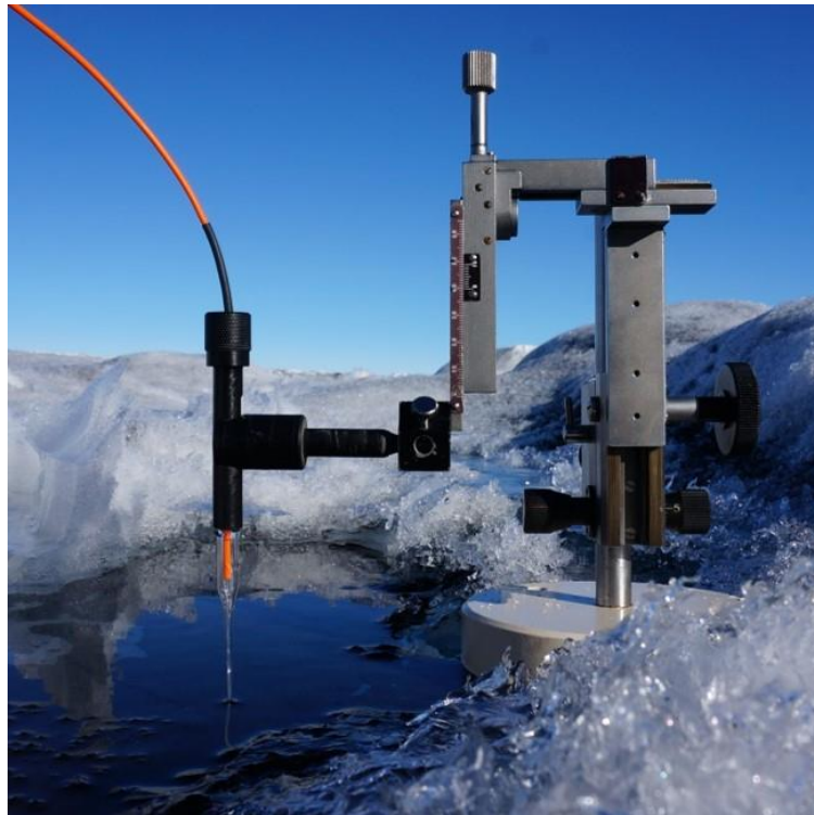
Figure 3.7. Measurement of oxygen profile in situ. Microoptode positioned with a manual micromanipulator for in situ measurement of an oxygen profile in a cryoconite hole on the surface of the Greenland Ice Sheet.
