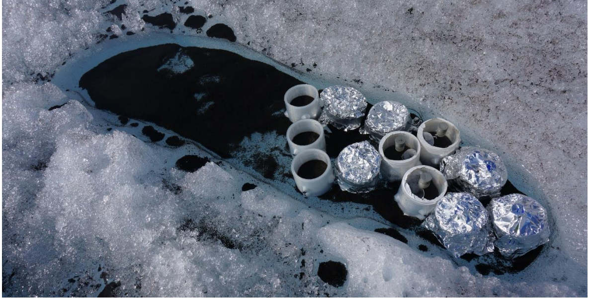
Figure 3.9. Cryoconite sediment incubations under in situ conditions. 3D-printed vessels incubated in a large cryoconite hole on Greenland Ice Sheet (2016).
