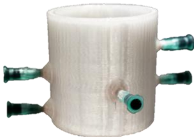
Figure 3.8. A custom-made incubation vessel, manufactured using 3D printing with sampling ports on the sides to enable measurement of oxygen, pH and microbial community changes with depth.
