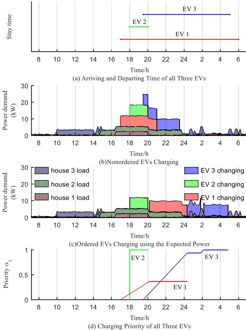
Figure 6.3 The EVs' charging process with the OCS using the expected power
