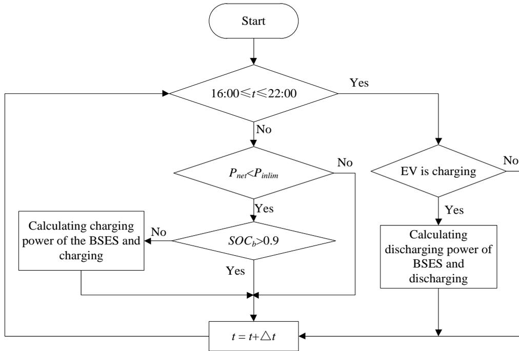
Figure 5.32 The Flow Chart of the BSES Operation with Limited Charging Time
