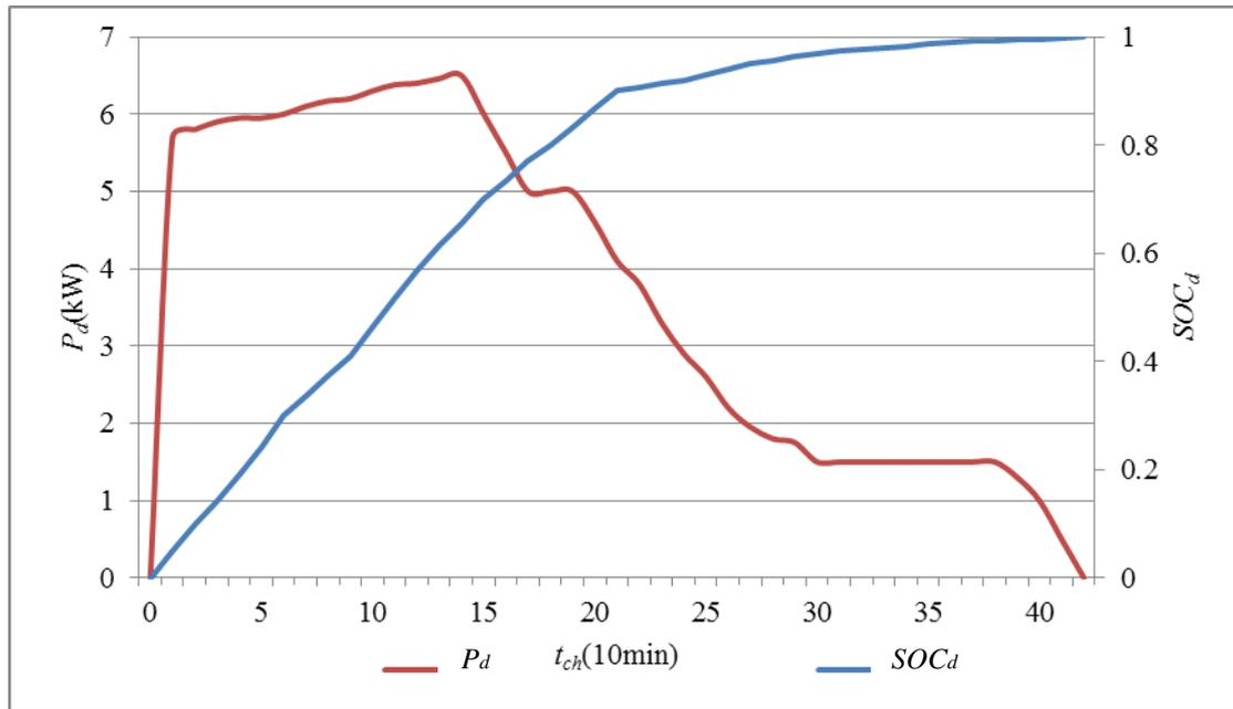
Figure 5.2 The SOC and Power Demand Profile of the Lead-acid Battery [127]
