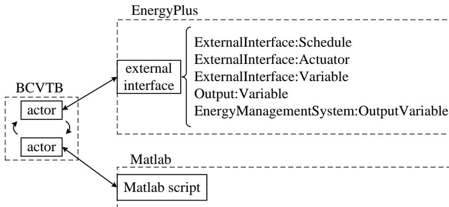
Figure 4.6 Interfaces Set up of EnergyPlus and Matlab
