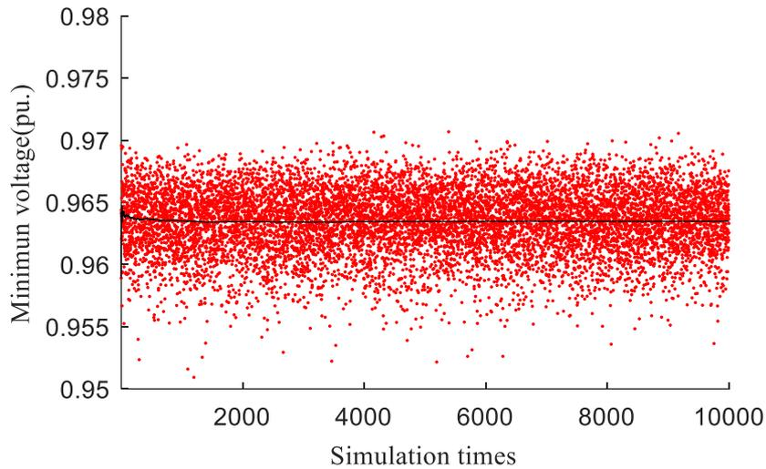
Figure 6.4 The Minimum Voltage of the Community Feeder with the OCS using the Expected Power
