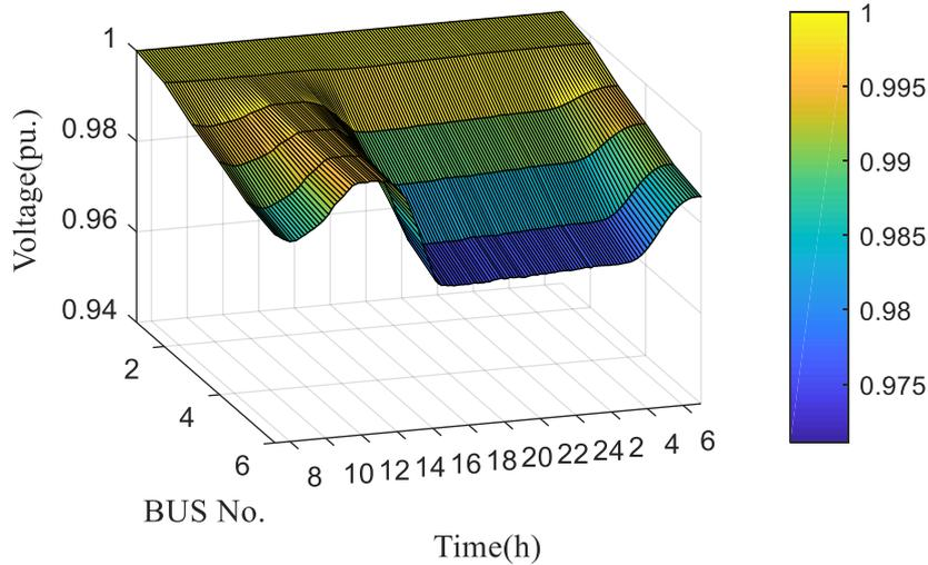
Figure 6.5 The Average Bus Voltage Distribution of the Community Feeder with the OCS using the Expected Power
