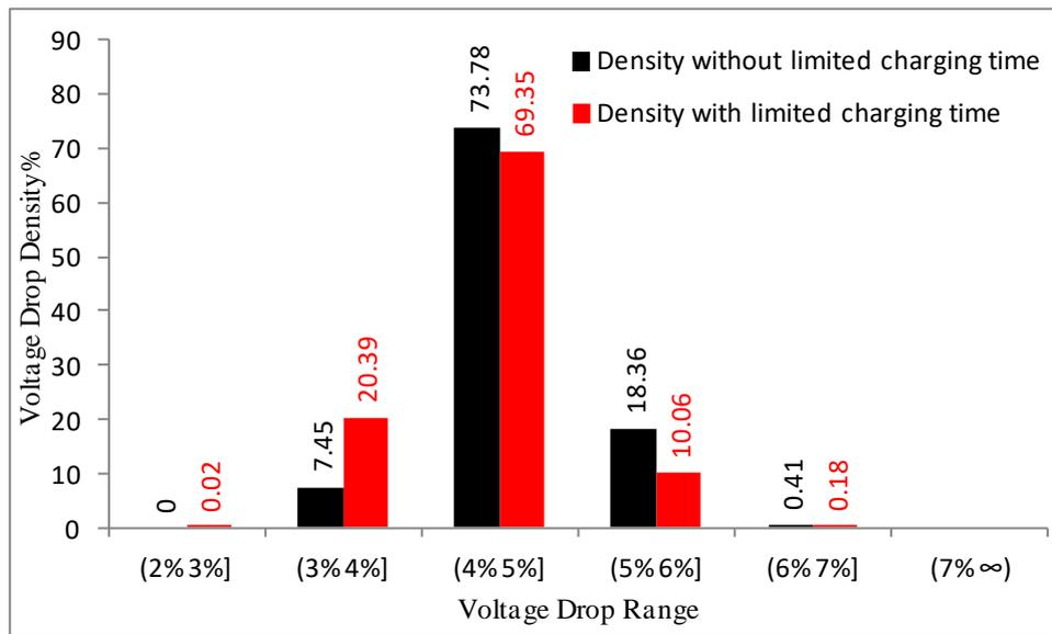
Figure 5.35 The Probability of Voltage Drop on BUS6 of the Community Feeder with Limited Charging Time
