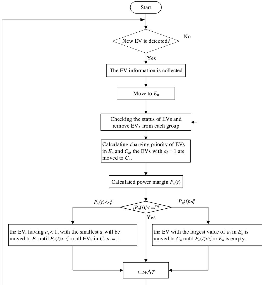
Figure 6.2 The Flow Chart of the OCS using the Expected Power
