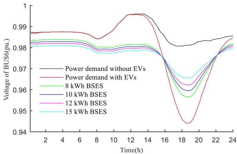
Figure 5.26 The Average Voltage on BUS6 of the Community Feeder with Different BSES Capacities.
