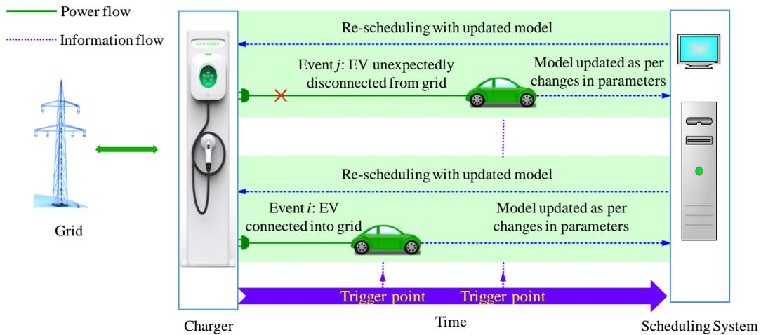
Figure 6.1 The Frame of Handling ‘Trigger Event’
