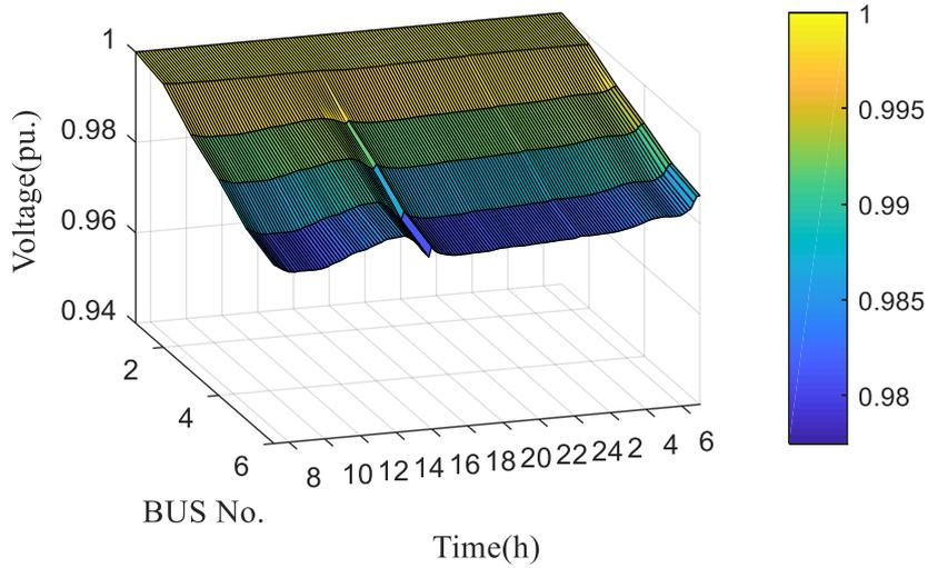
Figure 6.11 The Average Bus Voltage Distribution of the Community Feeder employing the OCS using Expected Power with the BSES
