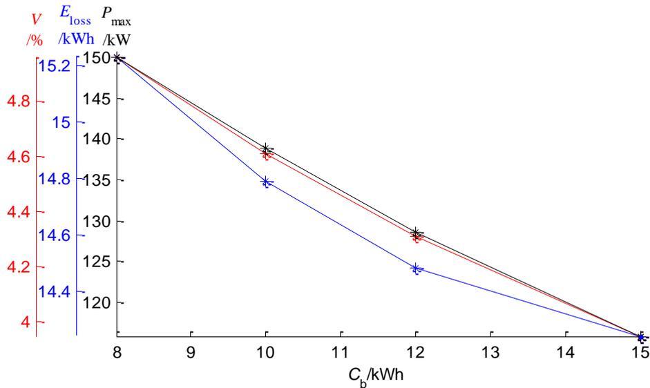
Figure 5.31 The Important Network Parameters under Different Capacities of the BSES
