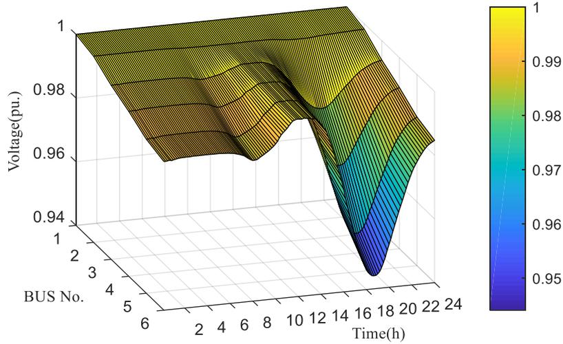
Figure 5.13 The Average Bus Voltage Distribution of the Community Feeder with EVs Charging
