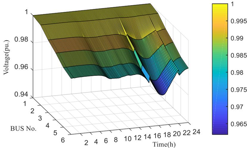
Figure 5.36 The Average Bus Voltage of the Community Feeder with Limited Charging Time of the BSES
