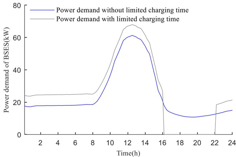
Figure 5.40 The Charging Power Demand of the BSES with Limited Charging Time of the BSES
