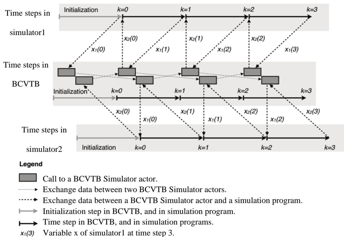
Figure 4.4 The Schematic Diagram of Data Exchange between Simulators and BCVTB [57]
