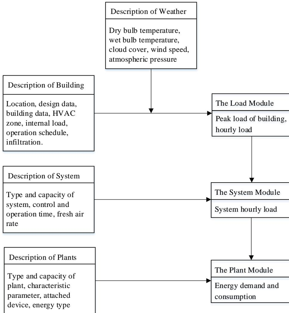
Figure 3.1 The Flow Chart of the Simulation Procedure in EnergyPlus[104]
