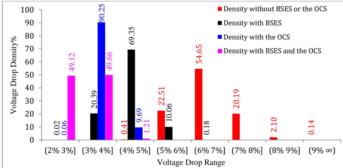
Figure 6.10 The Probability of Voltage Drop on BUS6 of Different Scenarios
