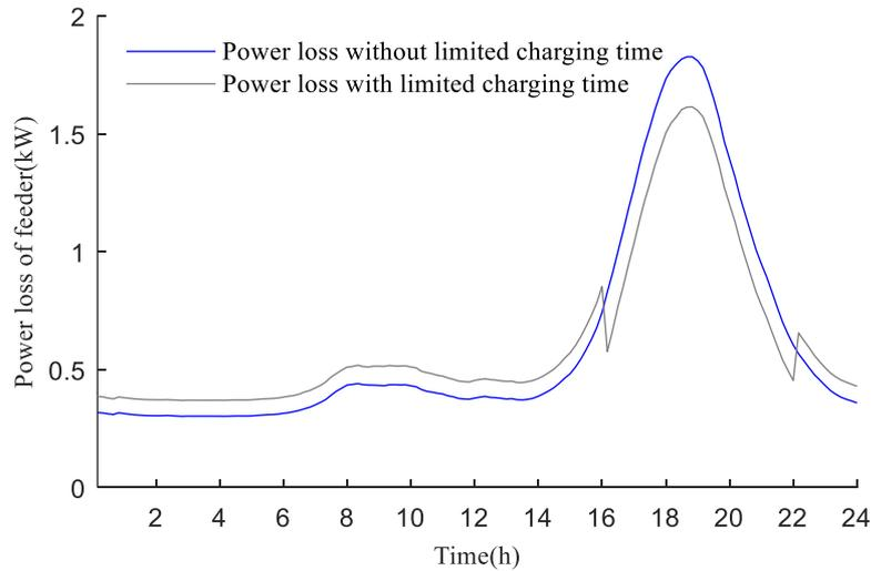
Figure 5.39 The Total Power Loss of the Community Feeder with Limited Charging Time of the BSES
