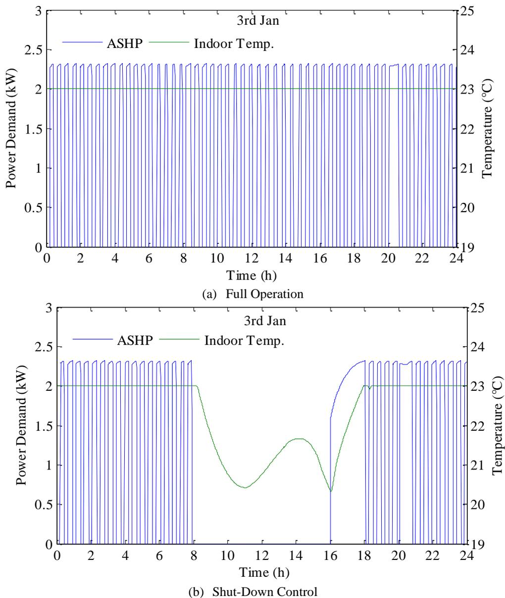
Figure 3.12 The Power Demand of the ASHP and the Indoor Temperature in the Dwelling on 3<sup>rd</sup> Jan
