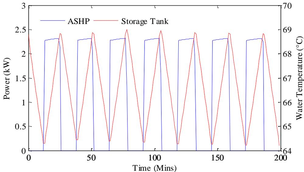
Figure 3.6 The Operating Relation Between the ASHP and Storage Tank
