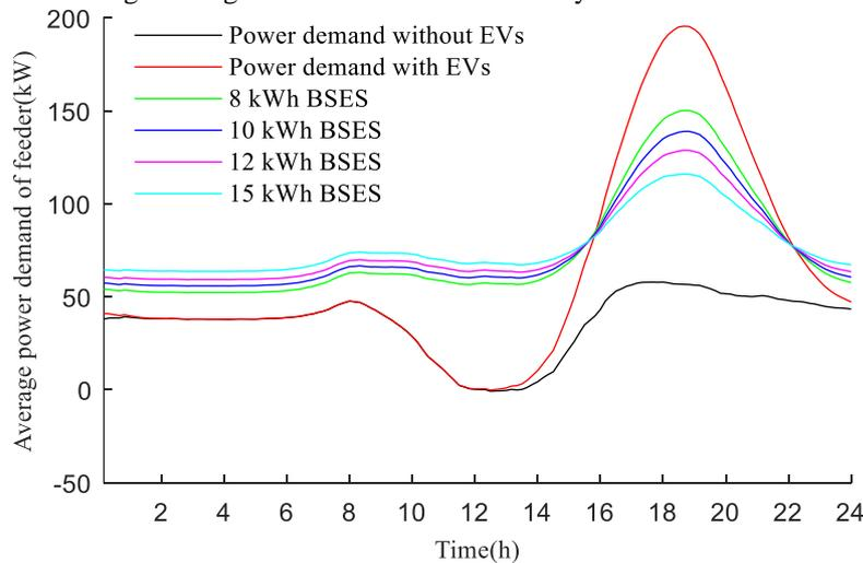
Figure 5.27 The Total Power Demand of the Community Feeder with Different BSES Capacities
