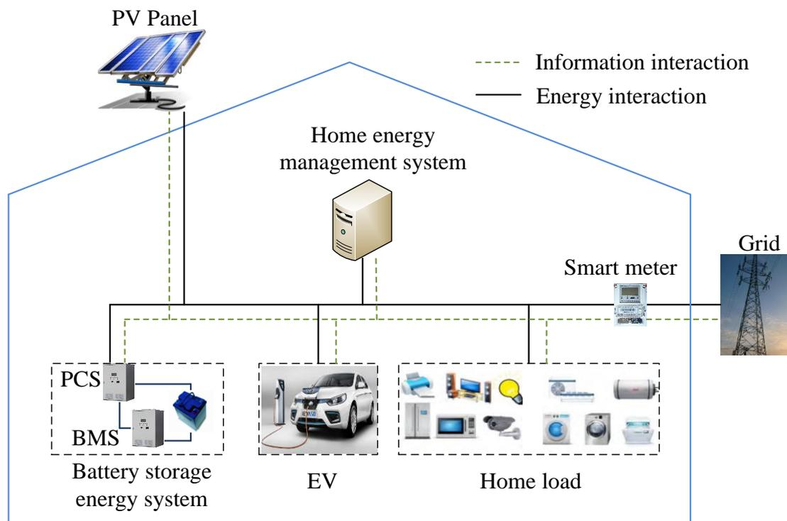
Figure 5.17 The Configuration of the Dwelling's Micro-grid.
