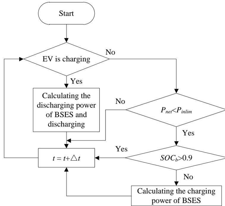
Figure 5.20 The Flow Chart of the BSES Operation.
