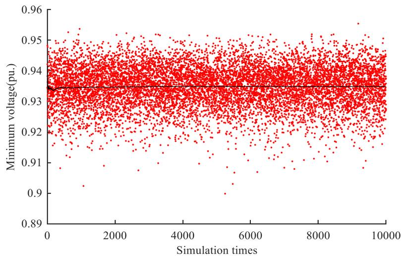
Figure 5.11 The Minimum Voltage along Simulation Times with EVs Charging
