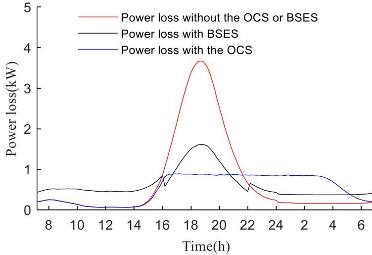
Figure 6.8 The Total Power Loss of the Community Feeder under Different Scenarios
