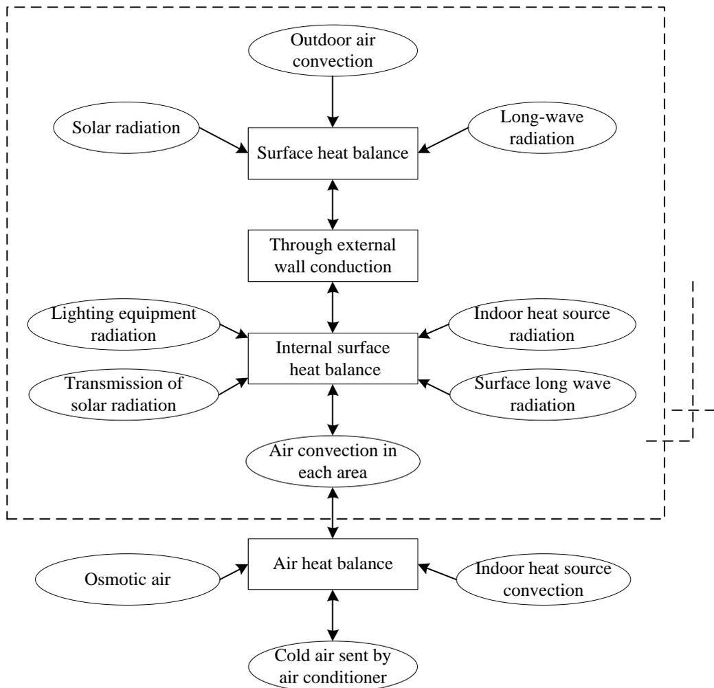
Figure 3.2 Schematic Diagram of the Heat Balance Method in EnergyPlus[105]
