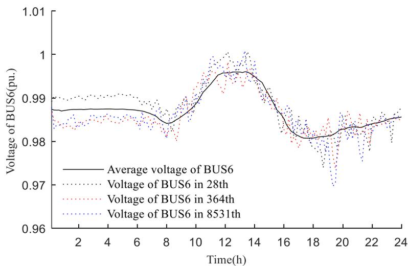
Figure 5.10 The Voltage on BUS6 of the Community Feeder without EVs Charging
