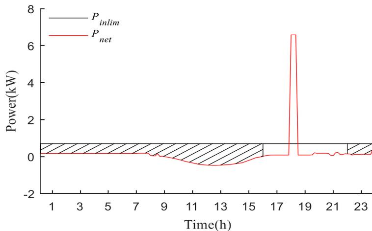
Figure 5.33 The Schematic Diagram of the Charging Process of the BSES with Limited Charging Time
