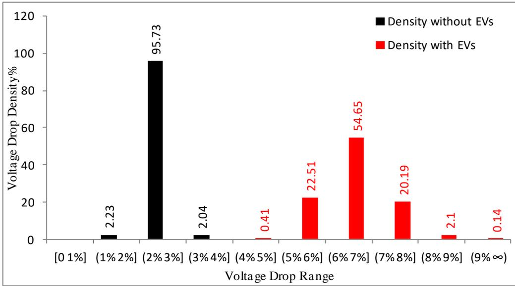
Figure 5.12 The Probability of Voltage Drop on BUS6 of the Community Feeder with/without EVs Charging
