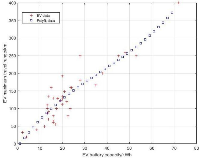
Figure 5.3 The Mathematical Relationship between EV Battery Capacity and Maximum Travel Range
