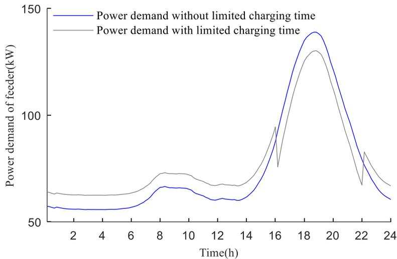
Figure 5.38 The Total Power Demand of the Community Feeder with Limited Charging Time of the BSES
