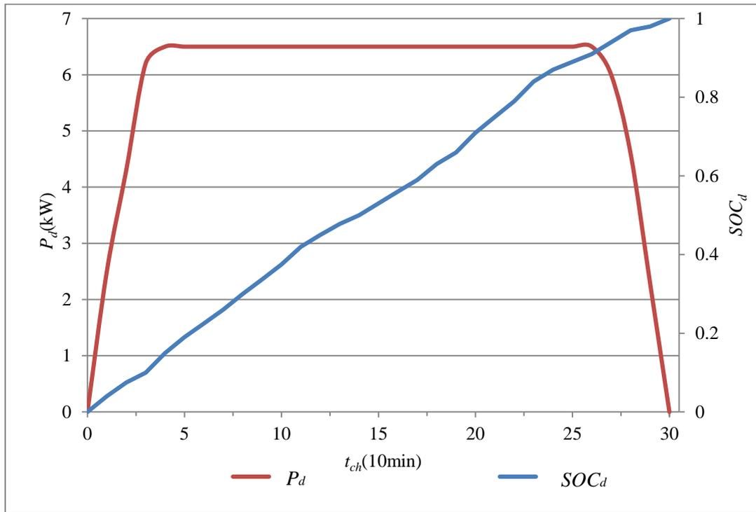
Figure 5.1 The SOC and Power Demand Profile of the Lithium-ion Battery [126]
