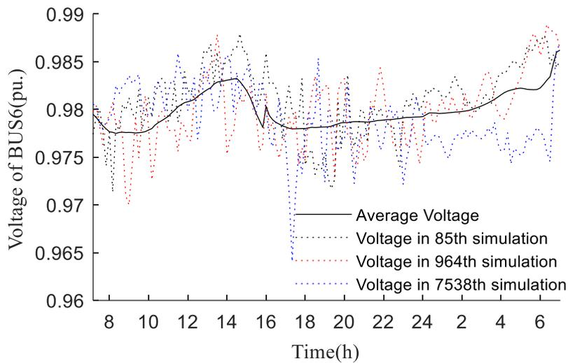
Figure 6.12 The Voltage on BUS6 of the Community Feeder employing the OCS using Expected Power with the BSES
