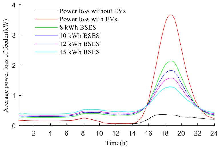
Figure 5.28 The Total Power Loss of the Community Feeder with Different BSES Capacities
