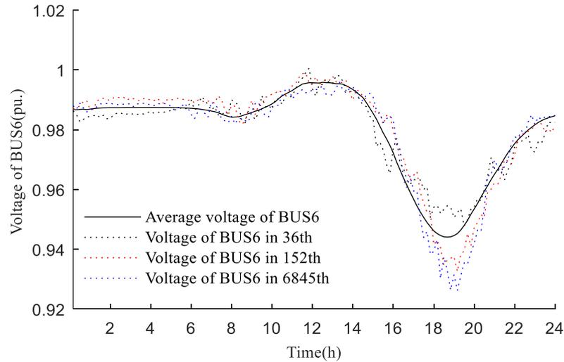
Figure 5.14 The Voltage on BUS6 of the Community Feeder with EVs Charging
