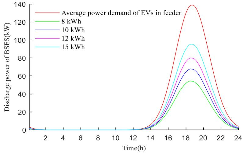
Figure 5.30 The Discharging Power Rate of the BSES
