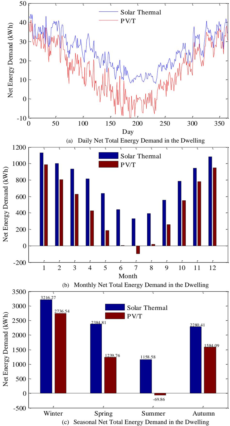
Figure 3.10 The Energy Demand in the Dwelling Separately with Solar Thermal Panel and PV/T Panels
