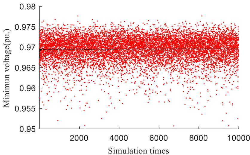
Figure 6.9 The Minimum Voltage of the Community Feeder employing the OCS using Expected Power with the BSES
