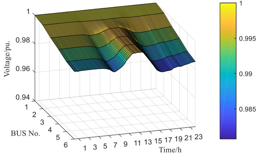
Figure 5.9 The Average Bus Voltage Distribution of the Community Feeder without EVs Charging
