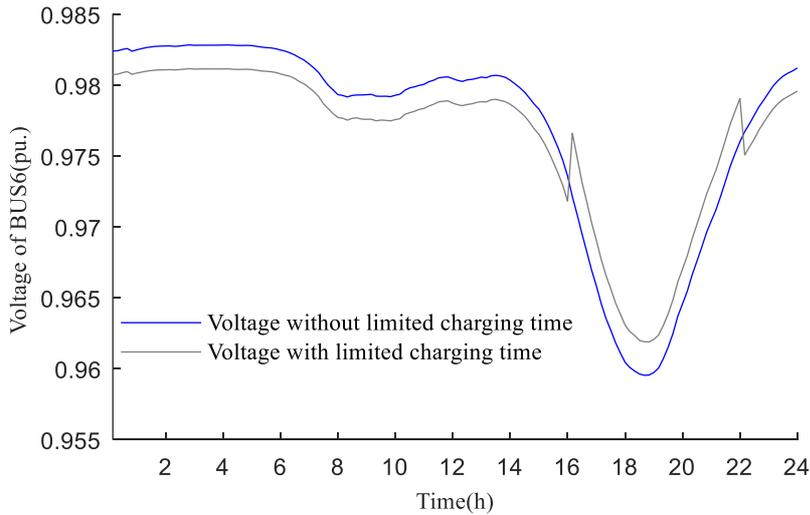
Figure 5.37 The Average Voltage of the BUS6 with Limited Charging Time
