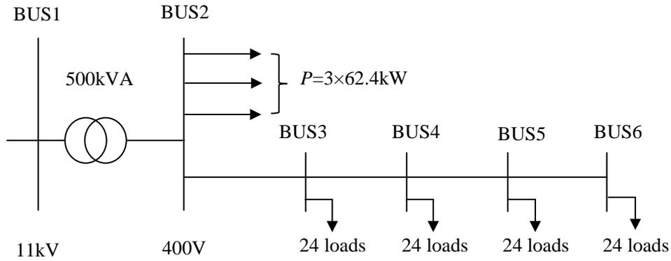
Figure 5.6 The Configuration of LV DN
