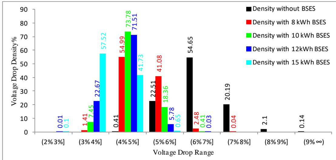
Figure 5.24 The Probability of Voltage Drop on BUS6 of the Community Feeder with Different BSES Capacities
