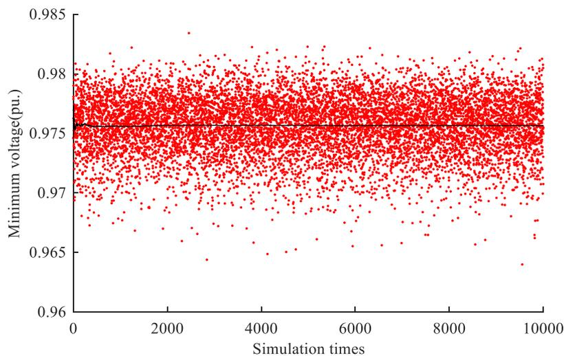
Figure 5.8 The Minimum Voltage along Simulation Times without EVs Charging
