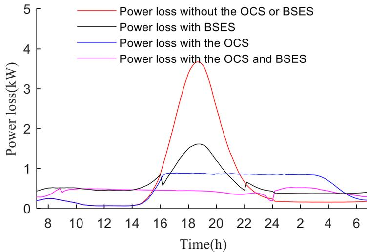
Figure 6.14 The Total Power Loss of the Community Feeder under Different Scenarios
