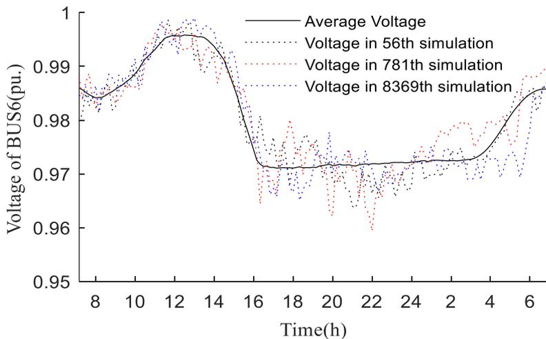
Figure 6.6 The Voltage on BUS6 of the Community Feeder with the OCS using the Expected Power
