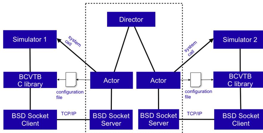
Figure 4.3 Architecture of the BCVTB[57]
