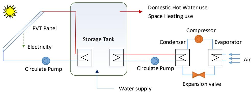
Figure 3.5 The Energy System of Electric Home
