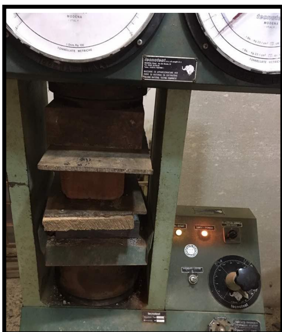
Figure 3.8, Image of compressive strength test on CEB
