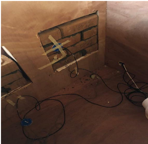
Figure 3.18: Internal view of the in-situ thermal test
