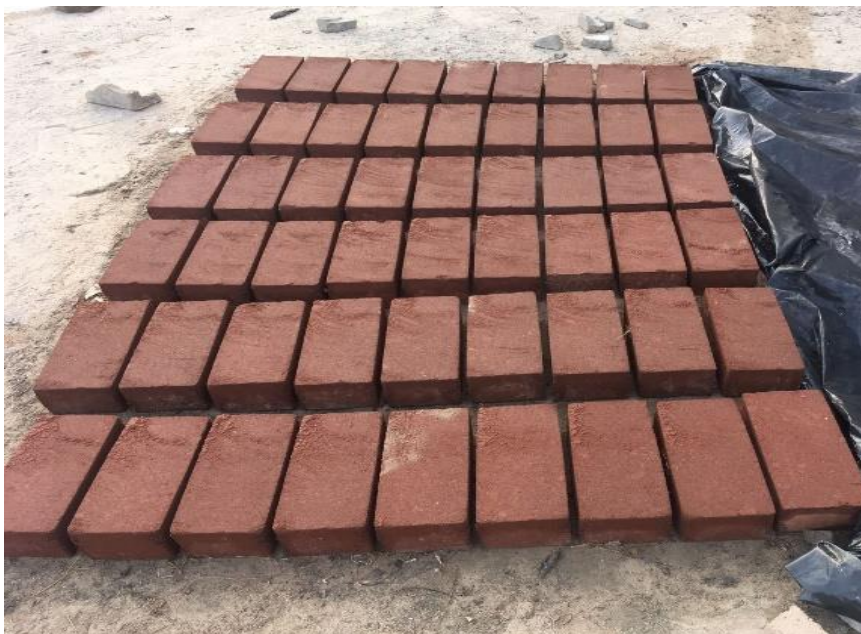
Figure 3.6. Samples of experimental solid CEBs produced in this study
