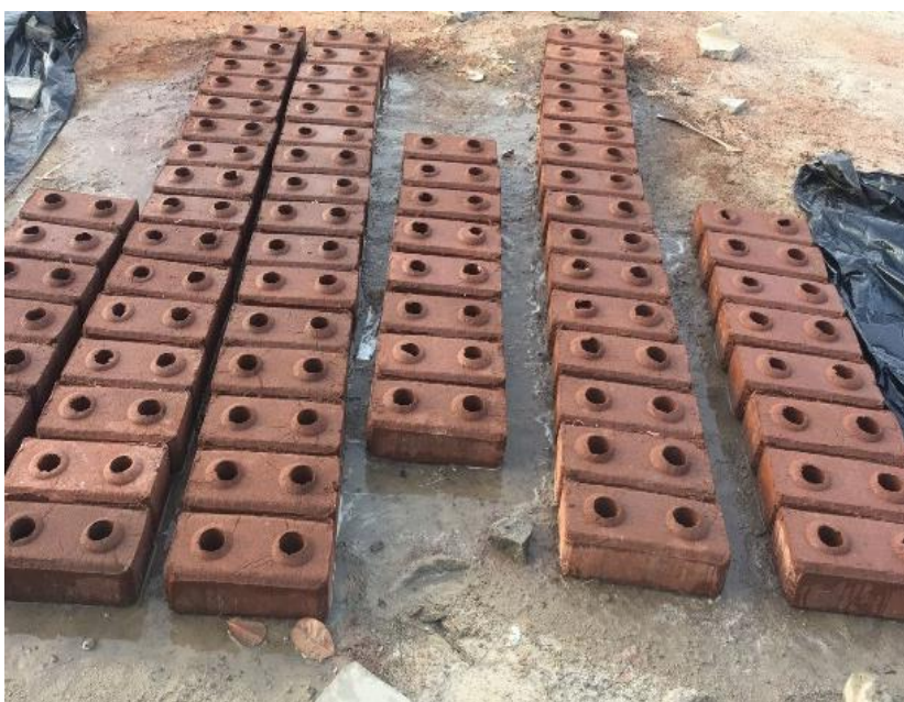
Figure 3.7. Samples of experimental hollow CEB produced in this study
