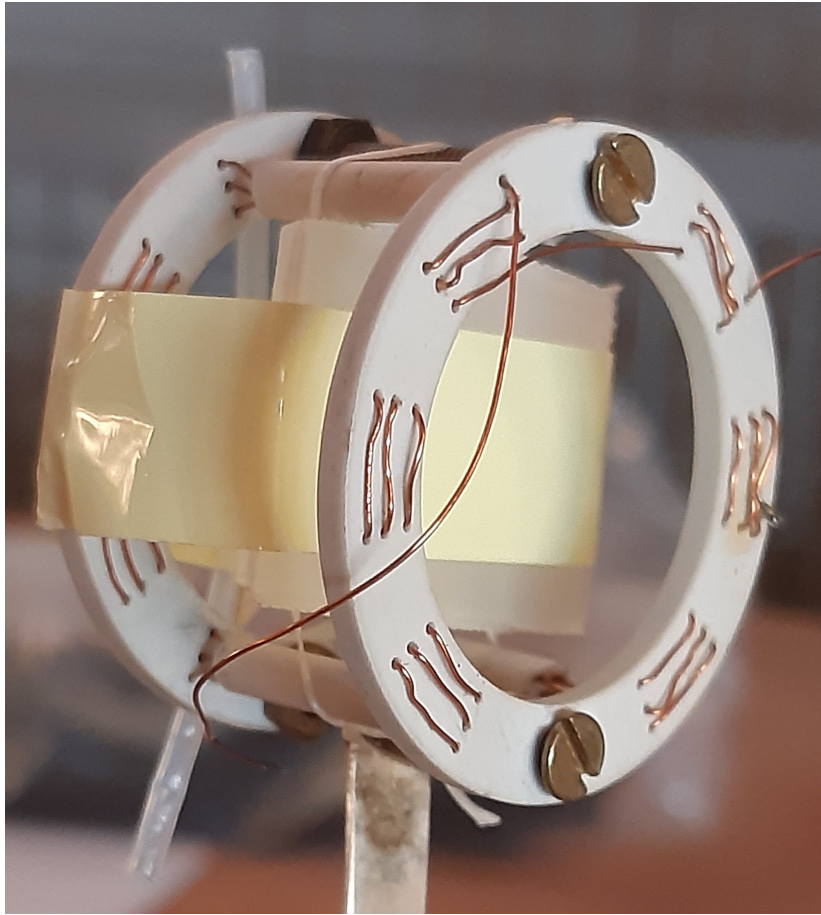
Figure 5.9: Photograph of the coil use to produce the RF field. The incoming muons arrive perpendicular to the white rings.
