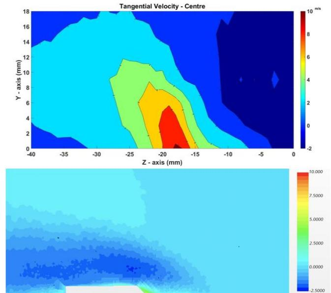
Figure 8 – Experimental (top) and numerical (bottom) profile of the tangential (j) velocity vector on the axial plane
