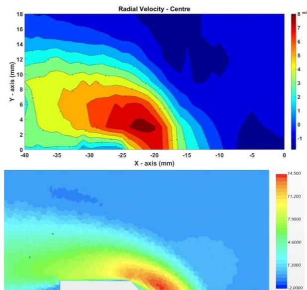
Figure 7 – Experimental (top) and numerical (bottom) profile of the radial (i) velocity magnitude vector on the axial plane
