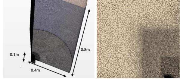
Figure 1 – generated mesh with computational domain and burner dimensions.
