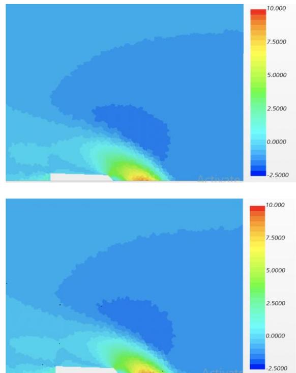
Figure 5 Numerical velocity profiles for axial planes cut at 10mm (top), 30mm (bottom) from the central plane
