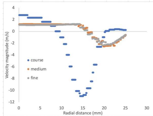
Figure 2 – Mesh sensitivity analysis
