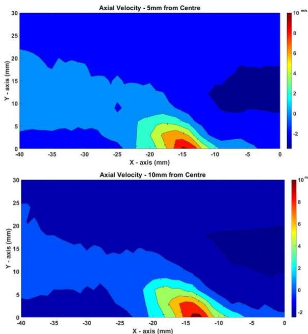
Figure 4 – experimental velocity profiles for axial planes cut at 5mm depth (top), 10mm depth (bottom)
