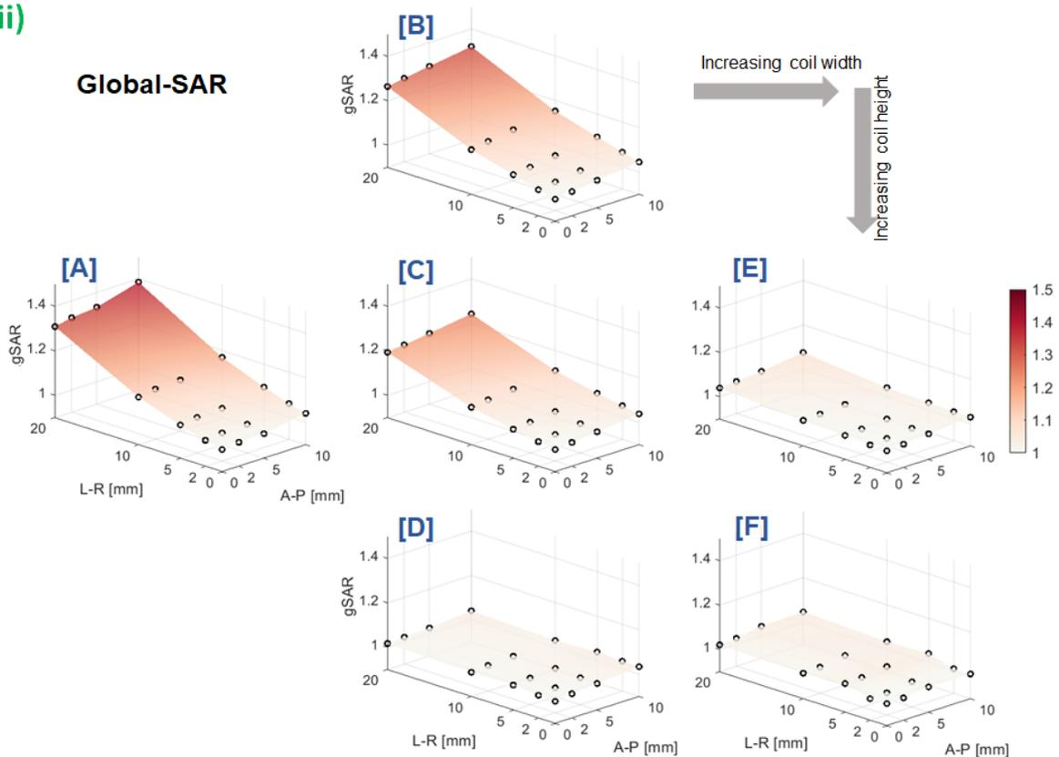
**Figure 2.** Motion-sensitivity of peak local-SAR (i) and whole-head SAR (ii) for RF-shim pulses designed using slice 2 at the central position for each coil model A to F. Slices 2-5 showed similar trends. Y-axes refer to SAR at each evaluated position (left-right [L-R] and anterior-posterior [A-P] displacements), as a factor of SAR at the central position (i.e. without motion).  $SAR_{\text{centre}}$  was comparable across coil models (not shown).
