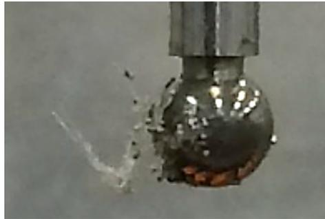
Figure 3.14. Collected probe debris after scanning measurement
