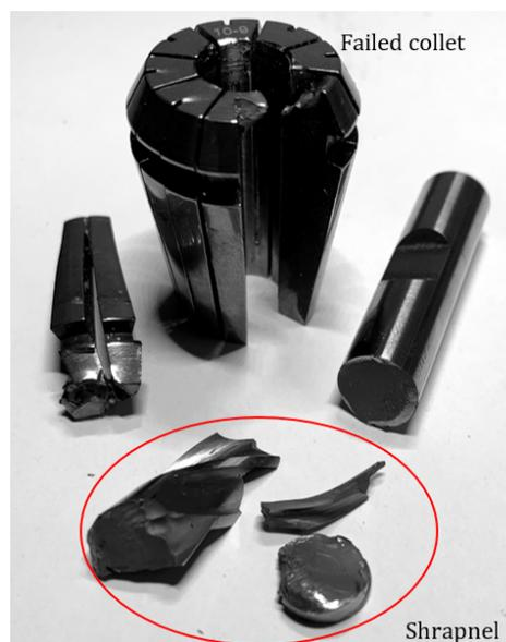
Figure 5.3. Disintegrated tool (catastrophic failure)
