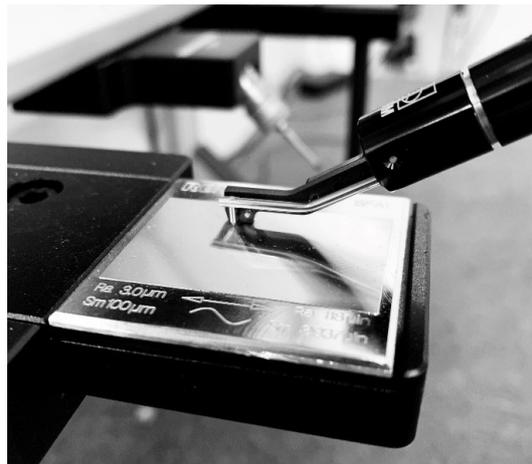
Figure 3.15. SFM-A2 acting on the  $3.0\mu\text{m}$  roughness specimen
