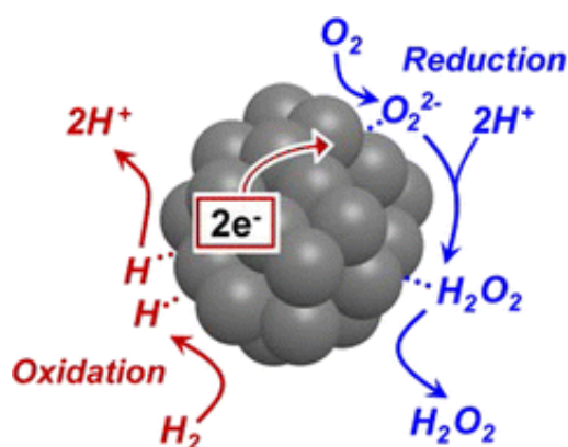
Scheme 1.3. Wilson et al. 's proposed mechanism of direct H_2O_2 synthesis over a Pd cluster via two half-reactions. Image adapted with permission from reference. 69 Further permission related to the material excerpted should be directed to the American Chemical Society (ACS).
