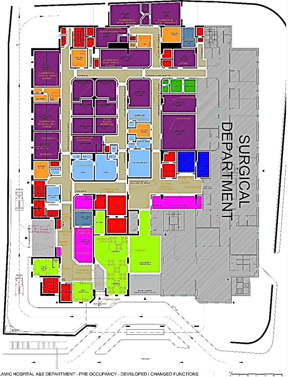
ISLAMIC HOSPITAL A&E DEPARTMENT - PRE OCCUPANCY - DEVELOPED / CHANGED FUNCTIONS TREATMENT / EXAM AREAS STAFF REST AREAS / MEETING ROOMS RADIOLOGY ENTRANCES DOCTORS & NURSES STATIONS/OFFICES PUBLIC AREAS ADMINISTRATION AND TRIAGE SURGERY DEPARTMENT PHARMACY LABORATORY CORRIDORS
