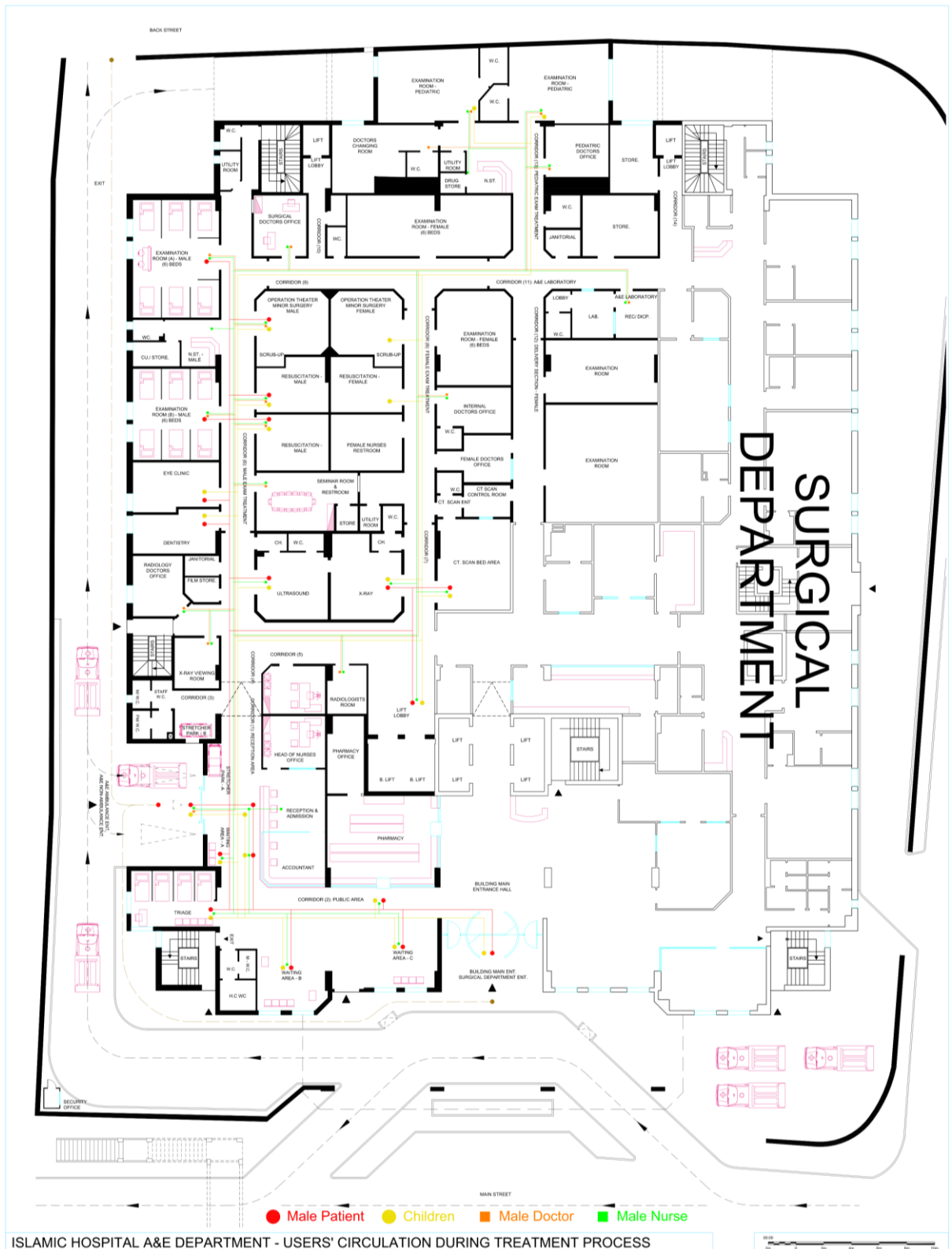
Figure 32: IH ED – patients’, nurses’, and doctors; movement paths to fulfil the clinical process.
