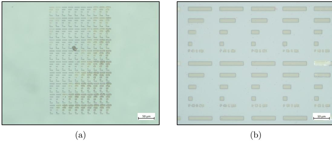
Figure 3.1: Optical microscopy images of cuboidal trenches with four different aspect-ratios in positive-tone photoresist. **a**, A dose array, laser power increases in 5% increments (left to right) and scan speed increases in  $3000 \mu m s^{-1}$  increments (bottom to top). **b**, Magnified view.
