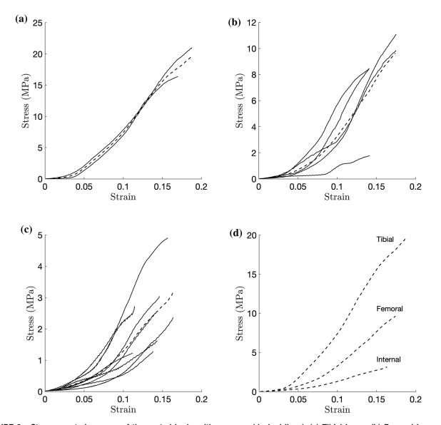
FIGURE 3. Stress vs. strain curves of the central body, with averages (dashed lines). (a) Tibial Layer; (b) Femoral Layer; (c) Internal Layer; (d) Averages.
