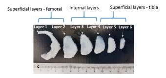
FIGURE 2. Results of the slicing process. It is possible to produce six to ten slices for each meniscus and differentiate between superficial and internal layers which have different mechanical behaviours.<sup>6</sup>
