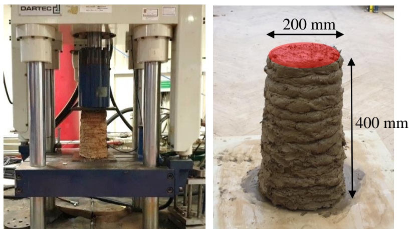
Figure 4: Compression test setup (left) and the cylindrical specimen (right).
