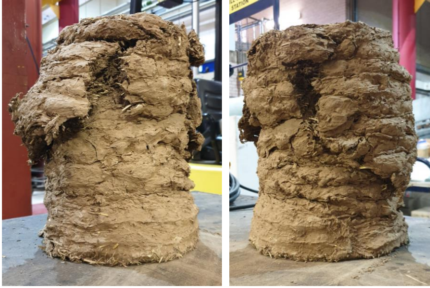
Figure 5: Typical examples of specimens after compressive failure.
