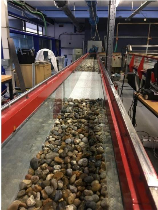
**Figure 4.8.** Overview, looking downstream, showing the placement of the artificial riverbed and gravel within the narrow flume in Cardiff University’s Hydro-Lab.
