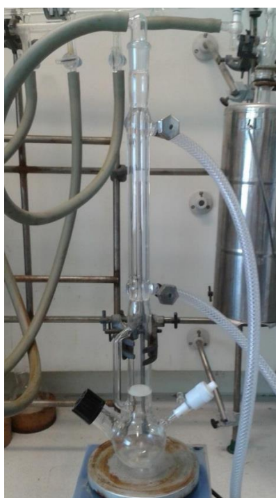
Figure 5.4: The Guerbet reactor used for open system alcohol coupling.
